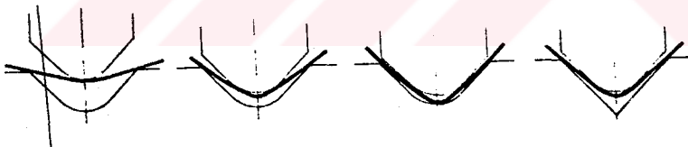
Figure 6. Shows 90^\circ V - die bending with large punch radius.
