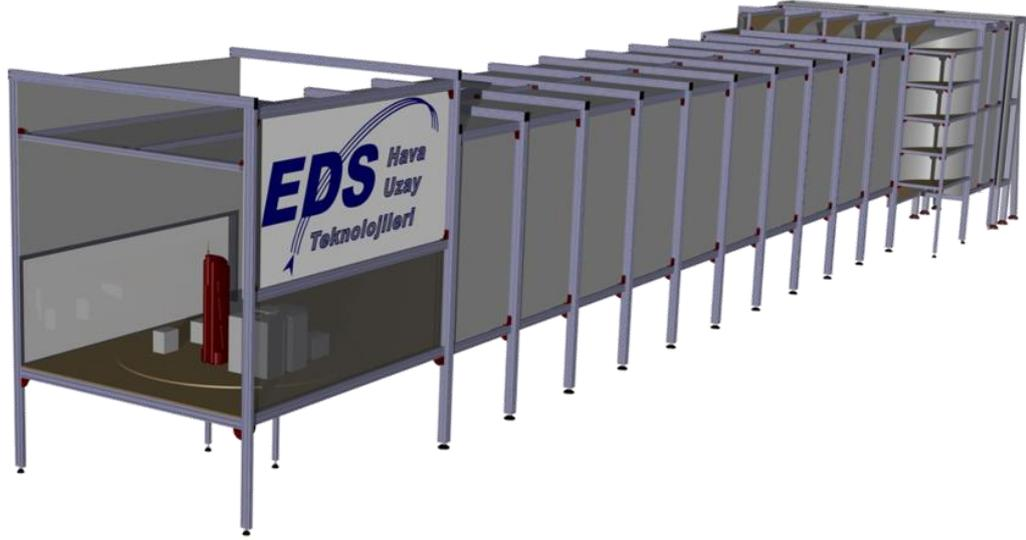
**Figure 1.8 :** EDS atmospheric boundary layer wind tunnel.
