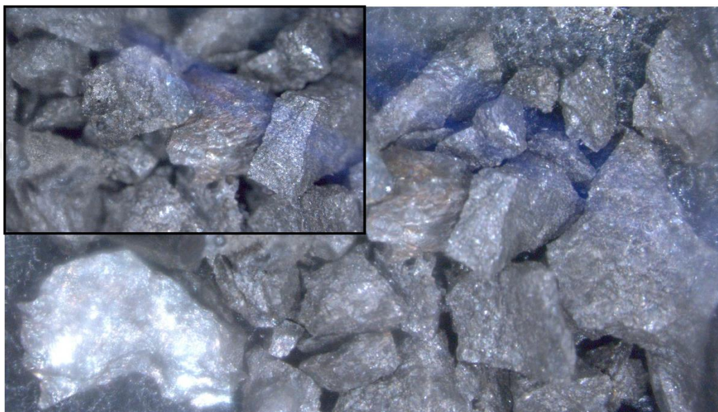
Figure 3.3: Optical microscope image of fayalite slag at x15 magnification. Inset shows image at x45 magnification.
