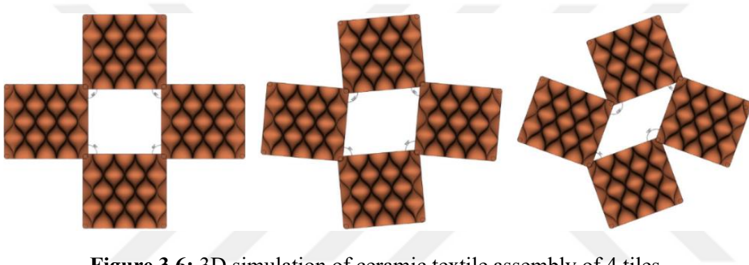
Figure 3.6: 3D simulation of ceramic textile assembly of 4 tiles.
