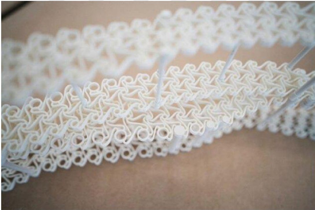
Figure 2.1: Parametrically designed auxetic pattern used for a shape-shifting wall at Hyperbody – Adapted from Albag, O. E. (2021).
