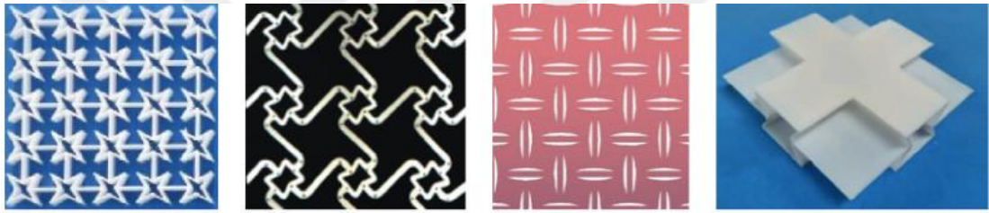
Figure 2.2: Classical auxetic metamaterials – Adapted from Zhao, C. (2025) .
