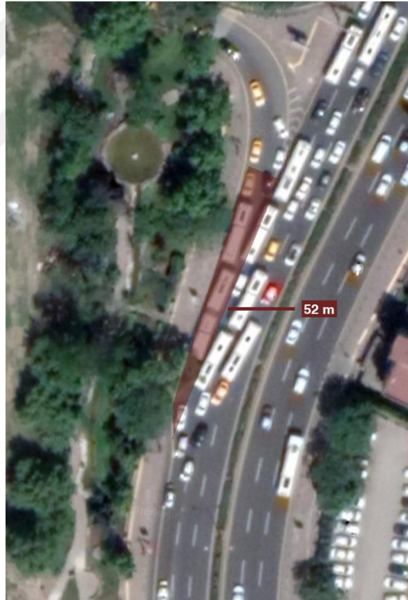
Figure 6.42 : The auxiliary lane that used as a parking lane at Talatpaşa Boulevard
