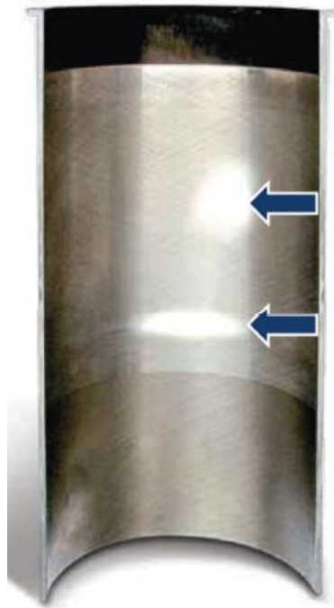
Figure 5.1 : Polishing due to local bore distortion [34].
