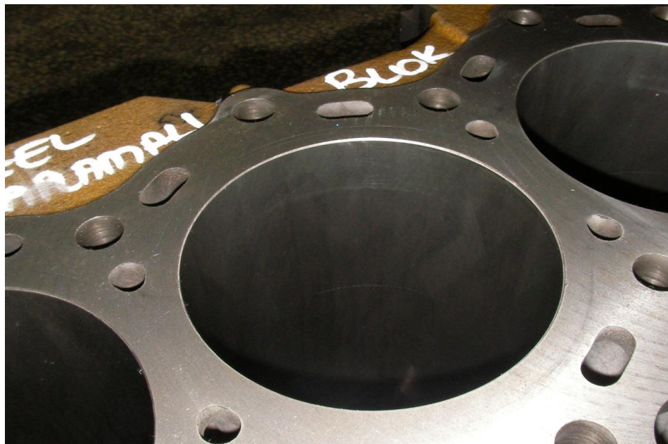
Figure 6.5 : BB49 Bore surface after honing.
