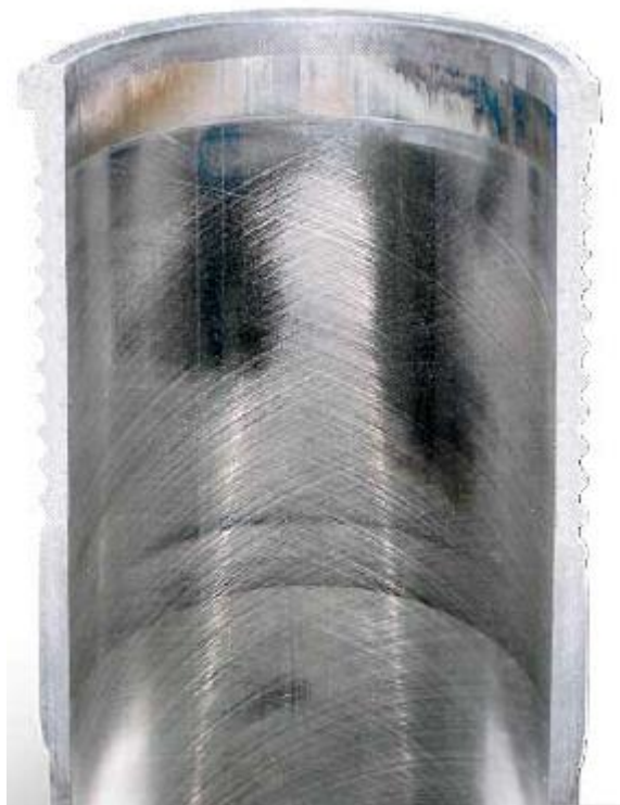
Figure 5.2 : Upper bore polishing [34].
