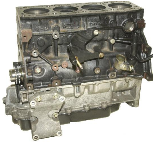
Figure 2.7 : Ford 1.8L lynx cylinder block with bedplate concept.
