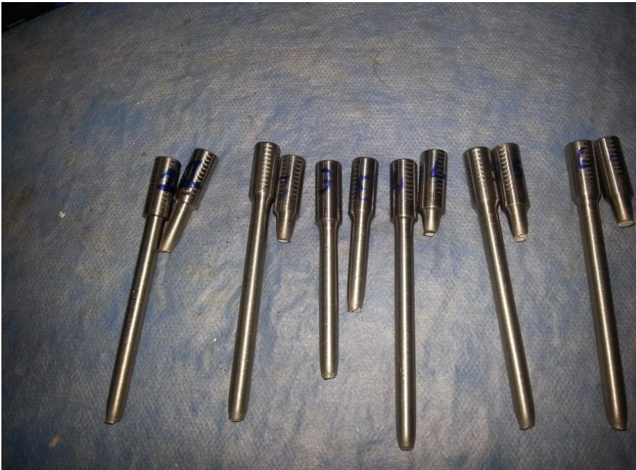
Figure 4.17 : AISI 1040 specimens after high temperature tests.
