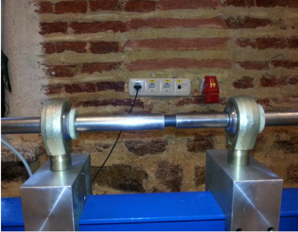
Figure 4.33 : AISI 1040 specimen for high strain rate testing.
