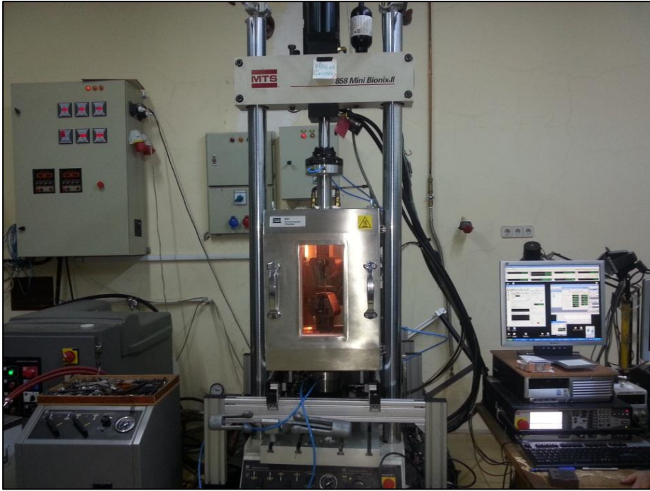
Figure 4.16 : Environmental chamber and data acquisition system.
