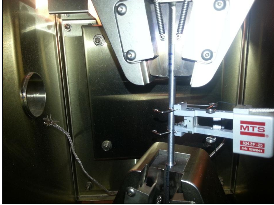
Figure 4.3 : Tensile test machine and MTS extensometer.
