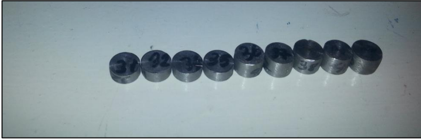
Figure 4.42: AISI 1045 test specimen after SHPB experiments.
