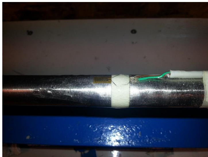
Figure 4.32 : Strain gage on the incident bar.
