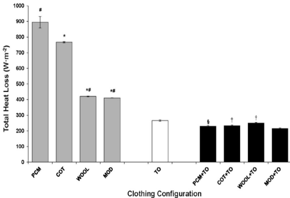
**Figure 1.4:** Total heat loss for different materials and ensembles. TO, turnout gear; PCM, phase change material; COT, cotton; MOD, modacrylic[49].
