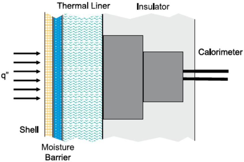
**Figure 1.3:** Measuring heat transfer in turnout systems[21].
