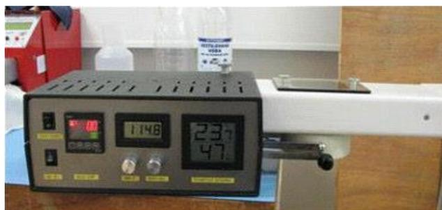
**Figure 4.2:** Permetest instrument.
