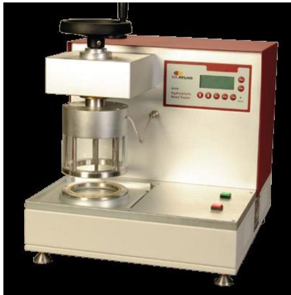
**Figure 3.9:** Photograph of hydrostatic head tester[30].
