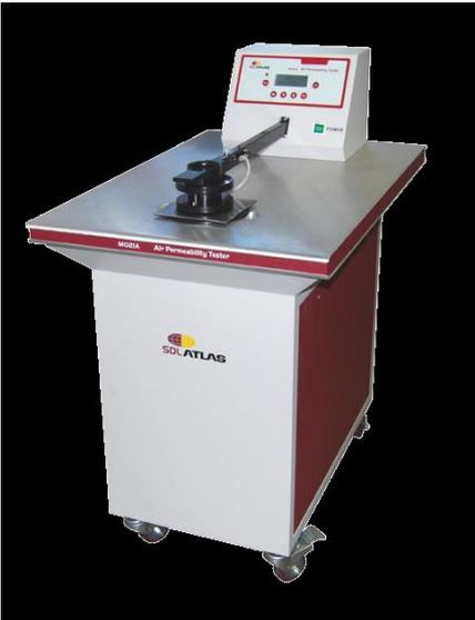
**Figure 3.10:** Air permeability tester[30].
