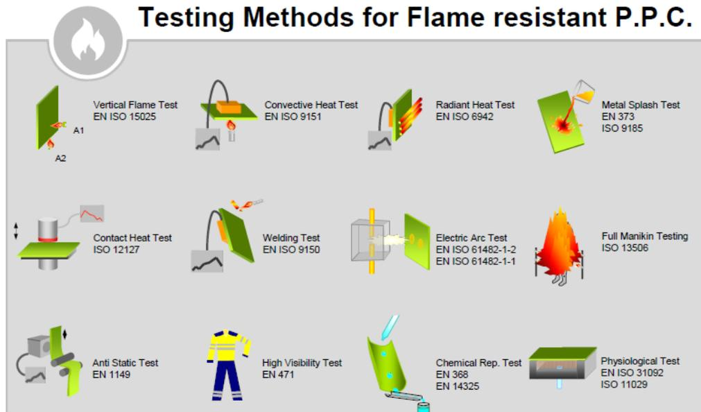
**Figure 3.1:** Testing methods for flame resistant personal protecting clothing [83].
