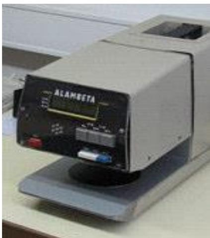
**Figure 3.7:** Photograph of Alambeta test instrument[27].
