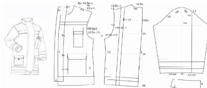
**Figure 2.1:** Construction and design of the protective jacket[61].
