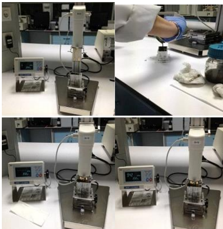
Figure 3. 6 : Image of the viscosimetry measurement process and the viscosimeter.
