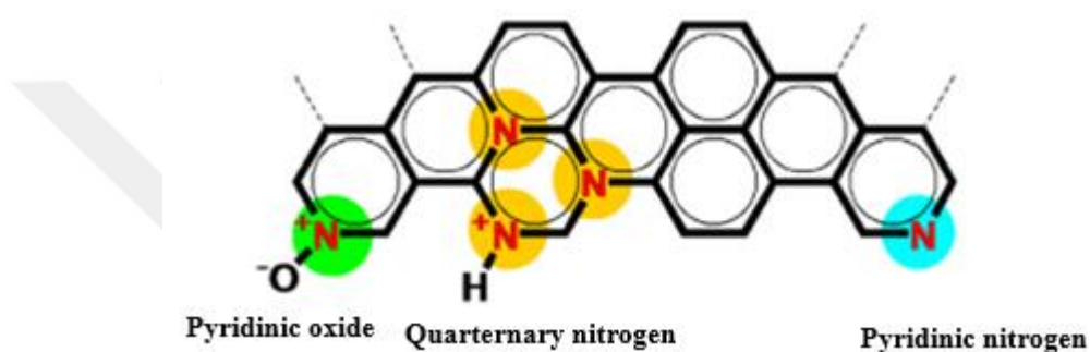
Figure 3.6 : Nitrogen species formed by post doping of CNT's [52].
