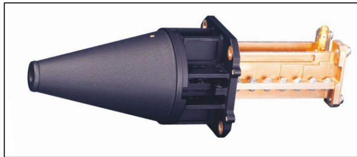
Figure 5.2 : Standby X-band antenna (RUAG Space)
