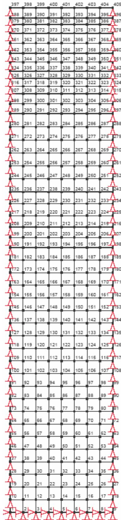
**Figure 6.35** Finite element mesh used in analysis including the imported soil profile from Bray et al (2004) (line 1)
