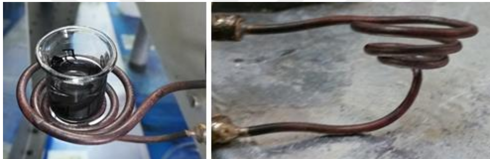
Figure 3.16 : Geometry of the helical coil that used in heating experiments.
