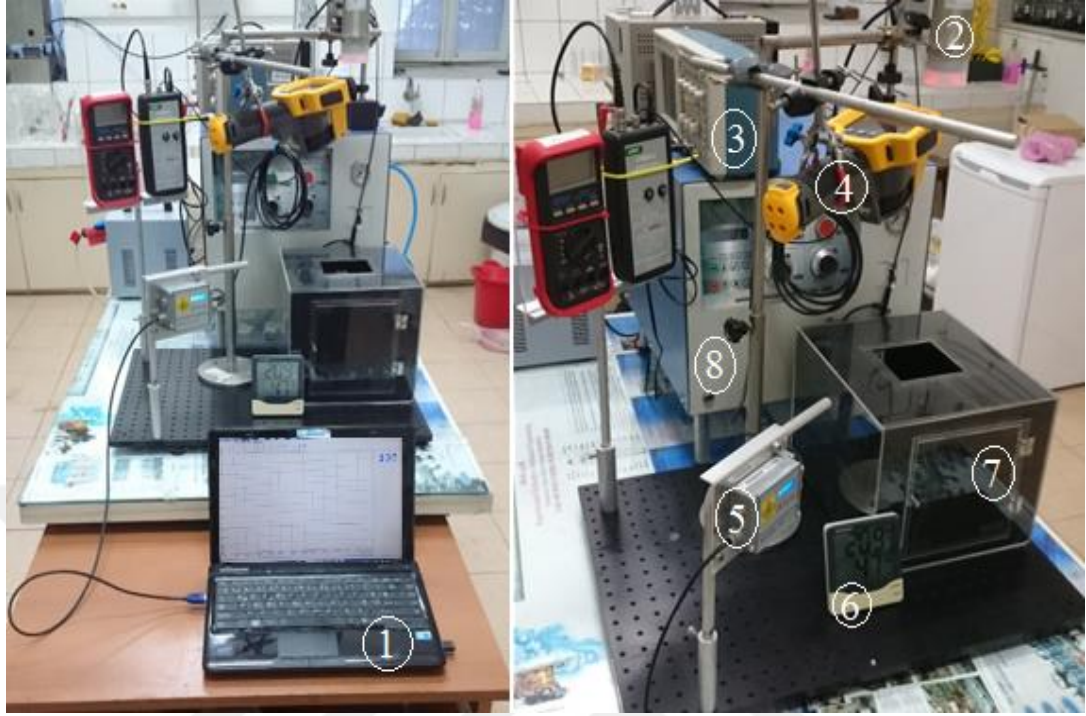
Figure 3.18 : Heating experimental set up with whole equipments: (1) Computer with Compact Connect Programme, (2) laser thermometer, (3) oscilloscope, (4) thermal camera, (5) PLC for laser thermometer, (6) thermometer, (7) black box for magnetic field and (8) induction generator.
