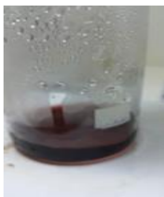
Figure 3.8 : Gold colloidal solution after added 1% (w/v) sodium citrate solution.
