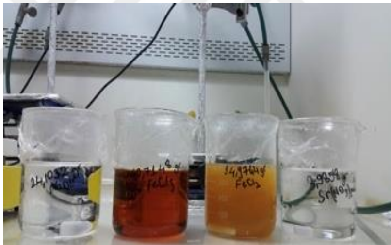
Figure 3.1 : The solution for core NPs synthesis from left to right respectively : \text{NaOH} , \text{FeCl}_3 , \text{FeCl}_2 , \text{Sr}(\text{NO}_3)_2 .
