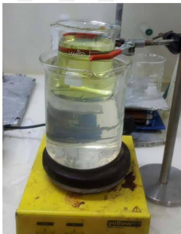
Figure 3.4 : Purification set up for H 2 AuCl 4 production.
