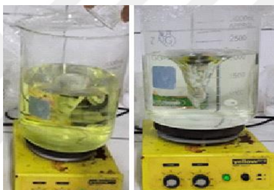
Figure 3.9 : Color change from pale yellow to transparent after added potassium carbonate solution on %1 \text{HAuCl}_4 .
