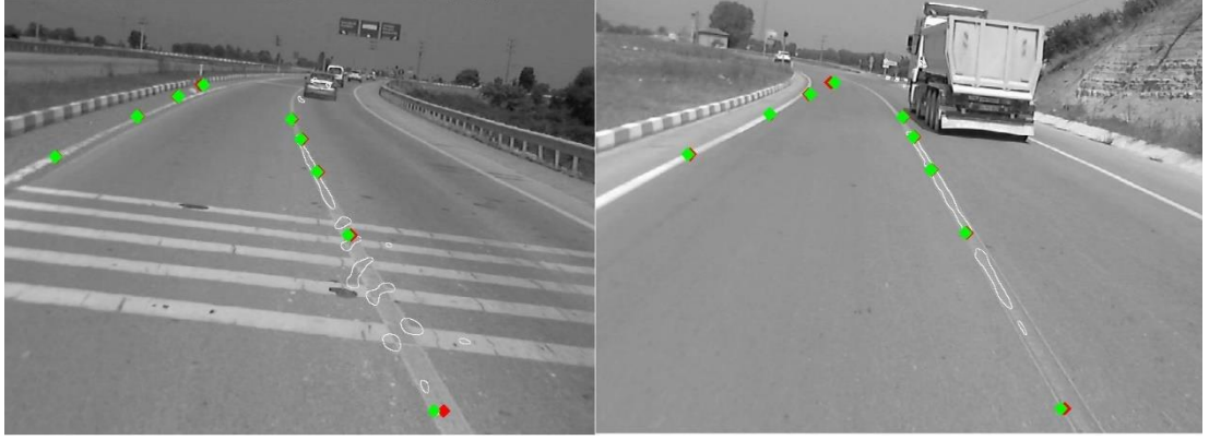
Figure 4.7 : Tracking algorithm results for curved roads.
