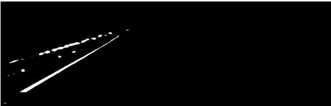
Figure 2.12 : Binary image after the intensity check.
