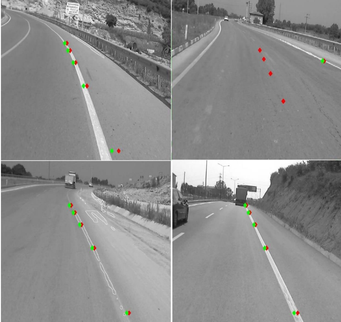
Figure 4.8 : Failure cases of the algorithm.
