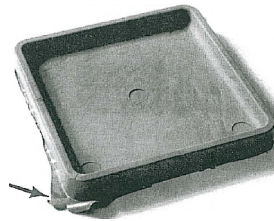
Figure 2.13 : Flashing due to over pressurization during mold filling [1].
