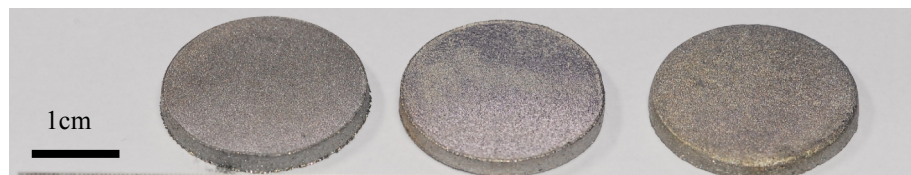
Figure 7.50 : The photo of isotropic injection molded and sintered parts, from left to right: F1-SSC, F2-VSC and F3-VSC.
