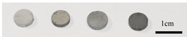
Figure 7.36 : The image of the sintered anisotropic single-pole F3-SNFB parts, from left to right: F3-SNFB-1 to F3-SNFB-4.
