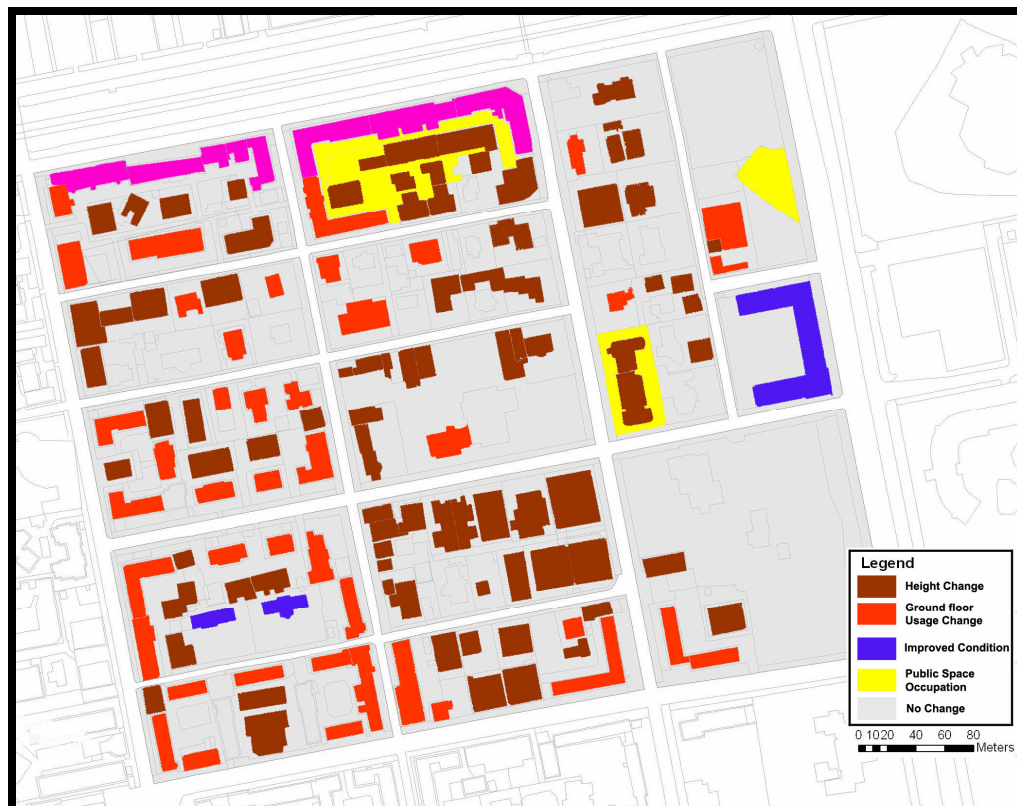
Figure 3.31 Synthesis of changes in the “Block” case study area
