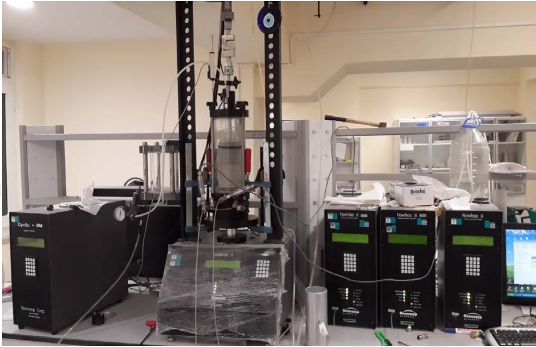
Figure 3.6 : Triaxial equipment used during experiments.
