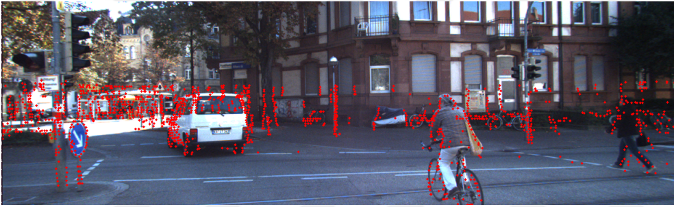
Figure 3.6 : Edged LiDAR point cloud on image.
