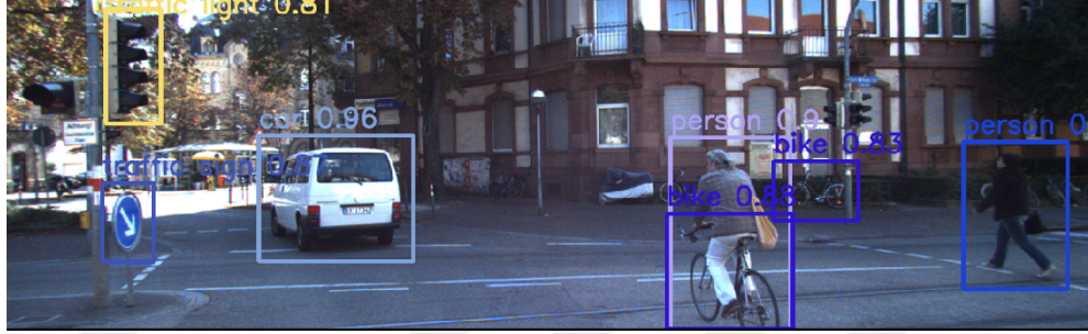
Figure 3.10 : YOLOv7-X object detections on the image.
