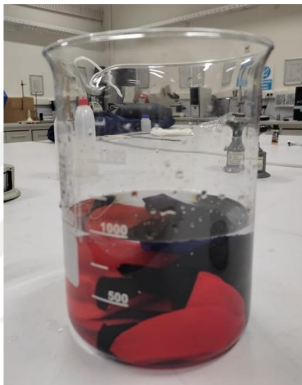
Figure 2.15.1: For drying rate test, Fabrics stay in distilled water for 30 min.
