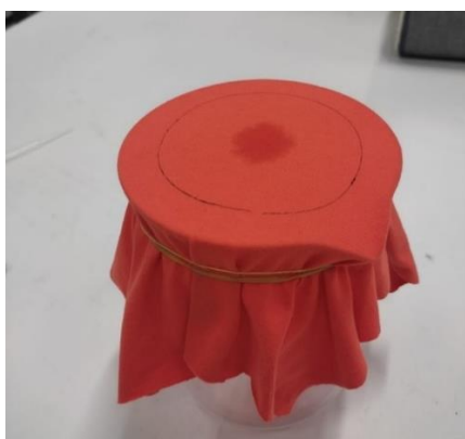
Figure 2.16.1.1 : After 6 th cycle, horizontal wicking test of Nm 30/1 60% cot 40% pet fabric.
