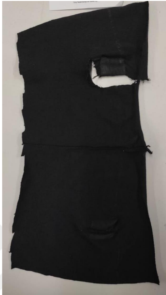
Figure 2.12.3 : 6 th cycle MCRP, after seam strength test. Fabric stitch is durable while fabric is broken.
