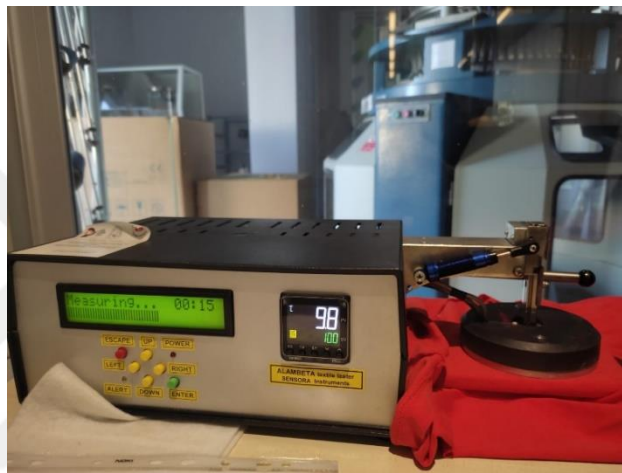
Figure 2.18.1: Thermal Conductivity Test from 3 rd cycle t-shirts.
