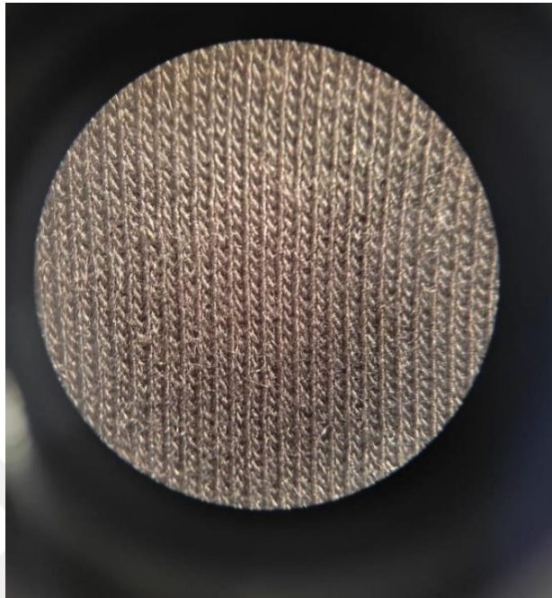
Figure-2.2.1: Nm 30/1 100% cotton fabric, at the end of 20000 cycles in abrasion (6 th cycle).
