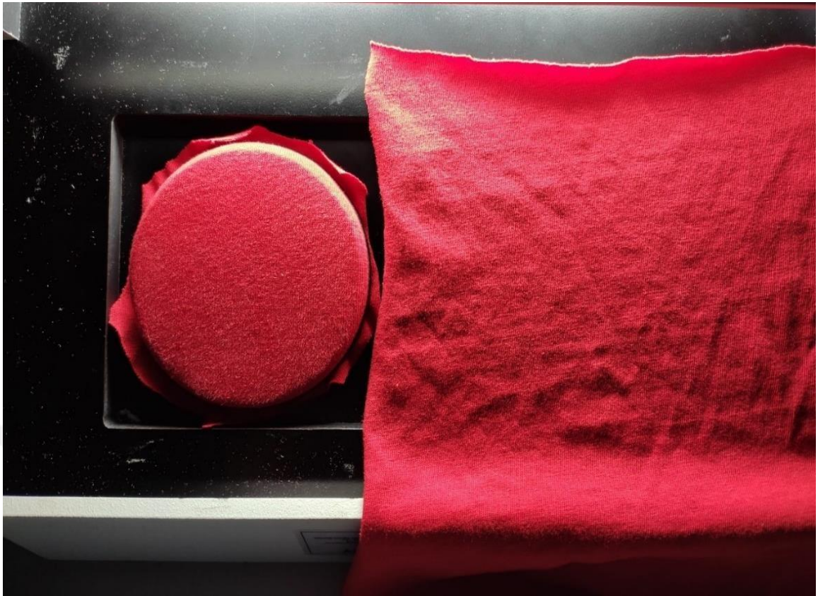
Figure-2.1.3.: Nm 20/1 40% preconsumer cot. 60% conventional cot. at the end of 7000 cycle in pilling (6 th cycle)
