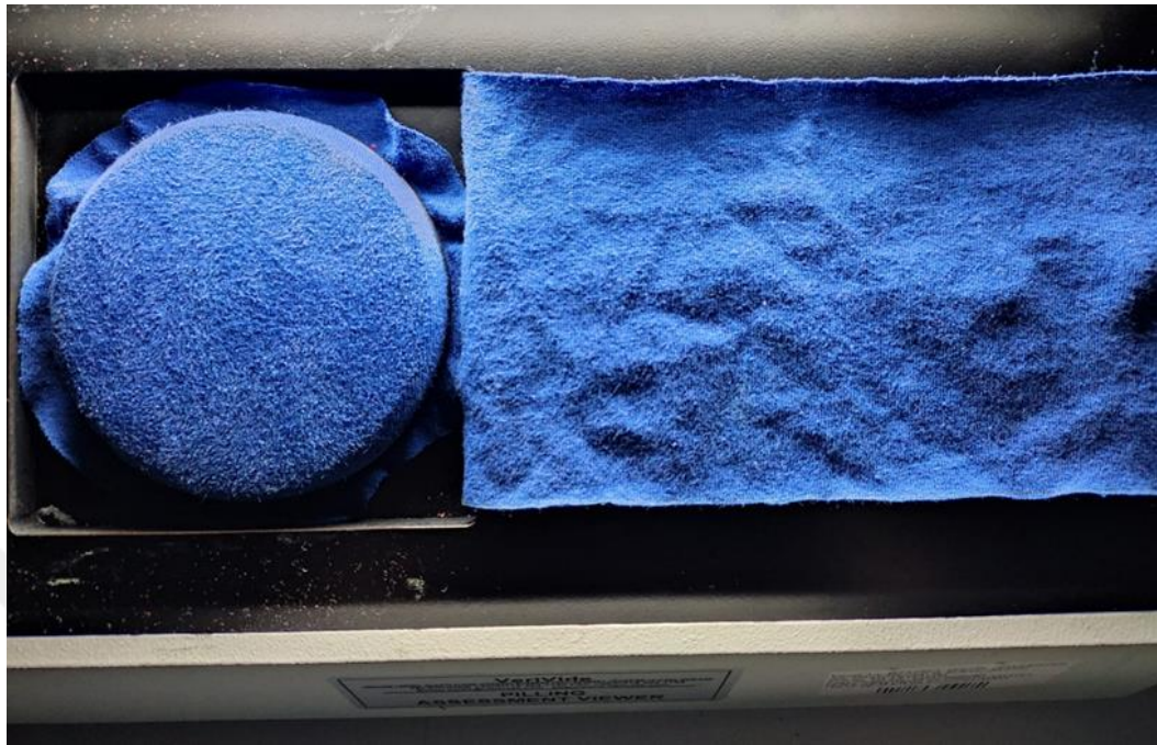
Figure 2.1.1 : Nm 20/1 100% recycle cotton fabric in color blue, end of 7000 cycles in pilling (6 th cycle).
