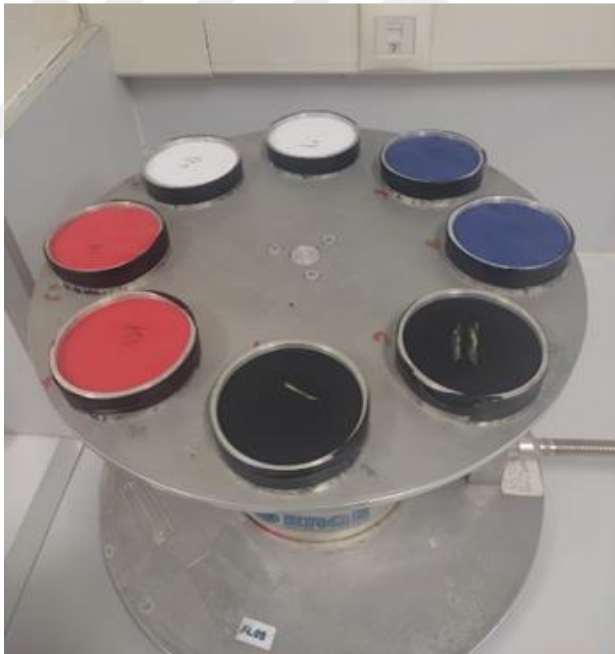
Figure 2.14.1.: Water vapour permeability testing.
