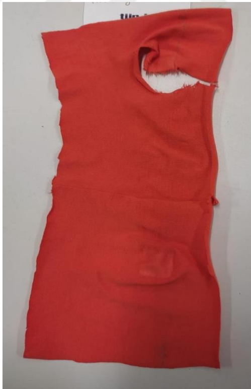
Figure 2.12.2 : 6 th cycle MCP, after Seam Strength test. Seam is maintained while fabric is broken.
