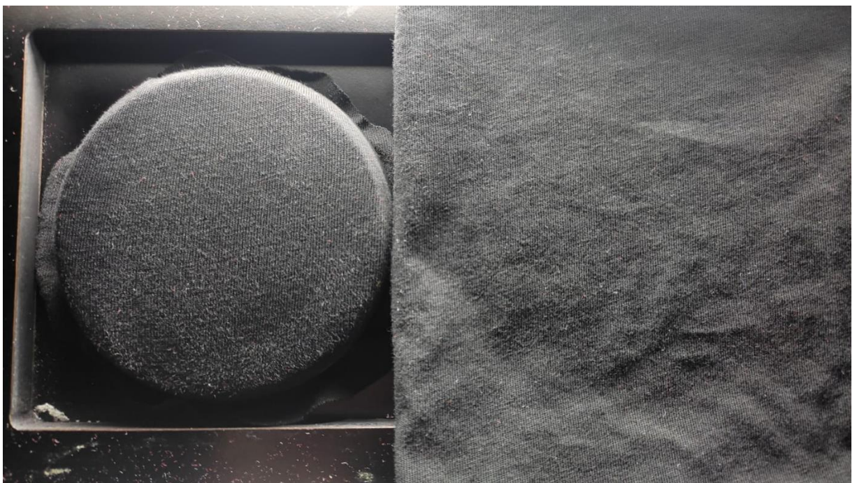
Figure-2.1.4.: Nm 30/1 100% cot. at the end of 7000 cycle in pilling (6 th cycle)
