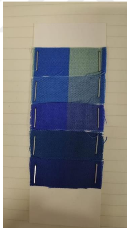
Figure 2.8.3.: Reference fabric for color fastness to light testing.
