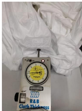
Figure 2.10.1 : Fabric thickness test of Nm 20/1 100% cot. fabric (After 3 rd cycle).
