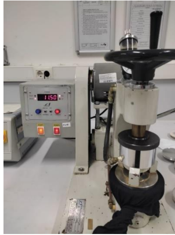
Figure 2.11.1: Bursting strength test of Nm 30/1 100%cot fabric (After 6 th cycle).
