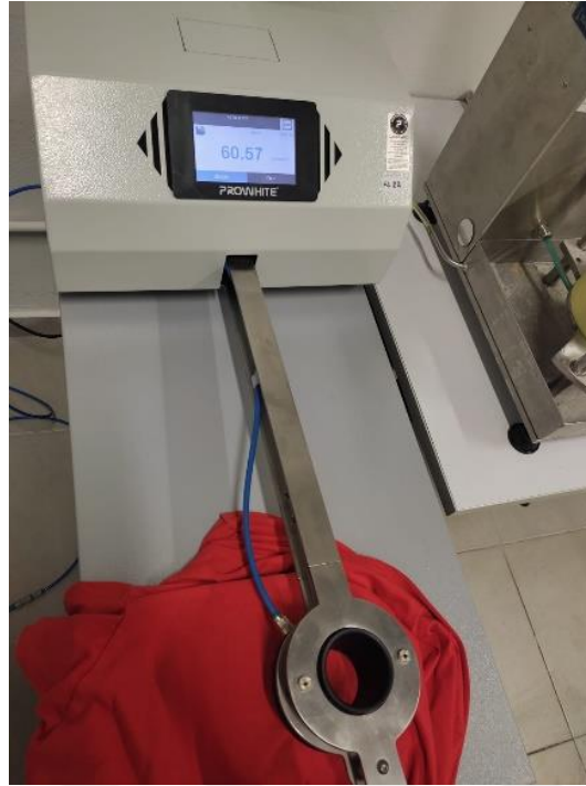
Figure 2.13.1.: Air Permeability Testing.
