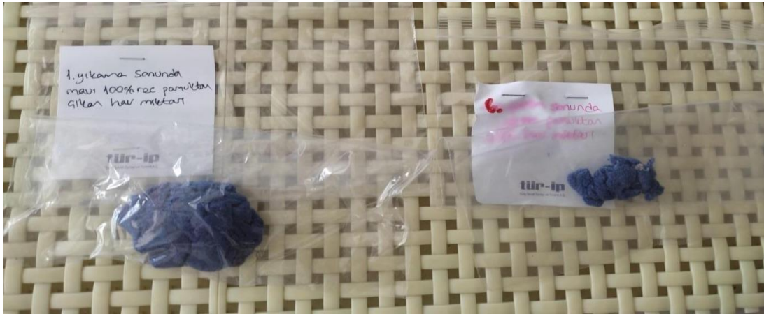
Figure 2.19.2 : Amount of fiber release of RC, at the end of 1 st & 6 th cycle.
