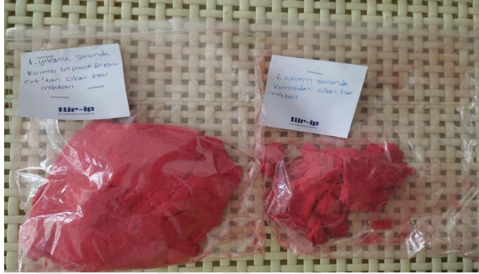
Figure 2.19.1 : Amount of fiber release of MCRC, at the end of 1 st & 6 th cycle.
