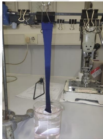
Figure 2.16.2.1: After 6 th cycle, vertical wicking test of Nm 20/1 100% rec. cot. fabric.
