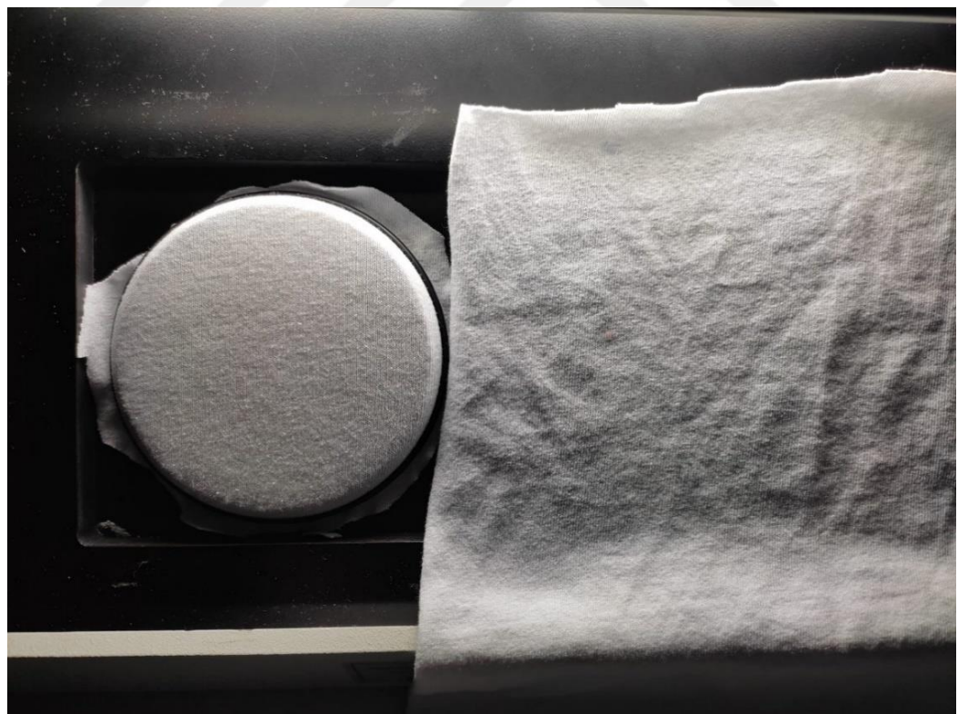
Figure-2.1.2.: Nm 20/1 100% cotton, at the end of 7000 cycles in pilling (6 th cycle).
