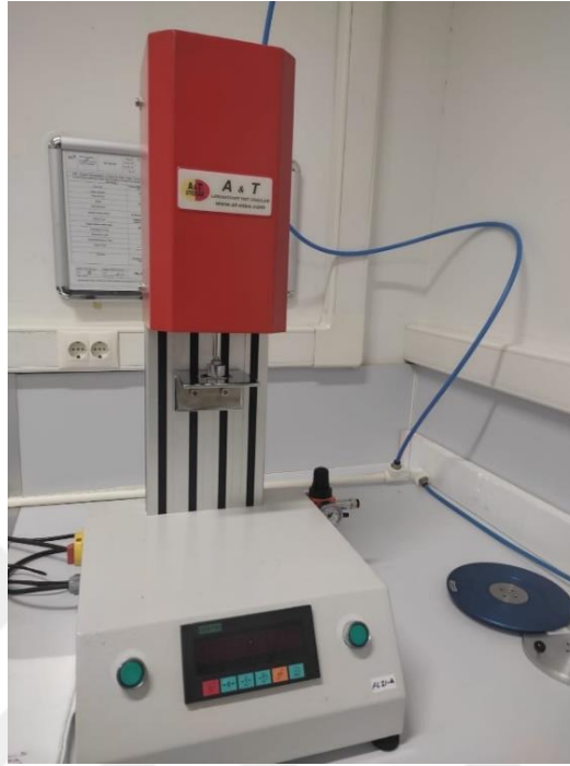
Figure-2.9.1: Fabric Stiffness Testing Machine.
