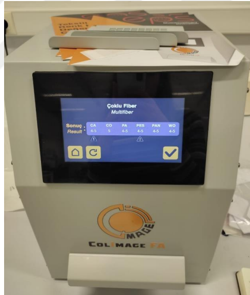
Figure-2.6.1.: Measurement machine for color fastness to washing test.
