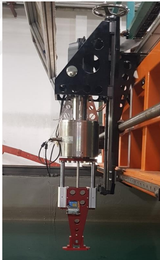
Figure 3.12 : Connection of loadcell and pantograph.
