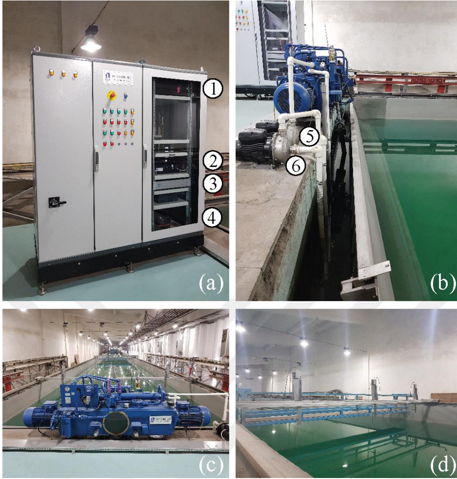
Figure 3.3 : The units of wave generator: (a) electrical control panel, (b) flap unit, (c) hydraulic unit, (d) wave probes and gauges. (1) computer, (2) Akamina – WaveGen Studio, (3) Tiab – Play waveform, (4) UPS, (5) coolant pump, (6) centrifuge pump.
