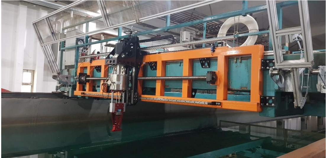
Figure 3.2 : Horizontal planar motion mechanism at Istanbul Technical University.
