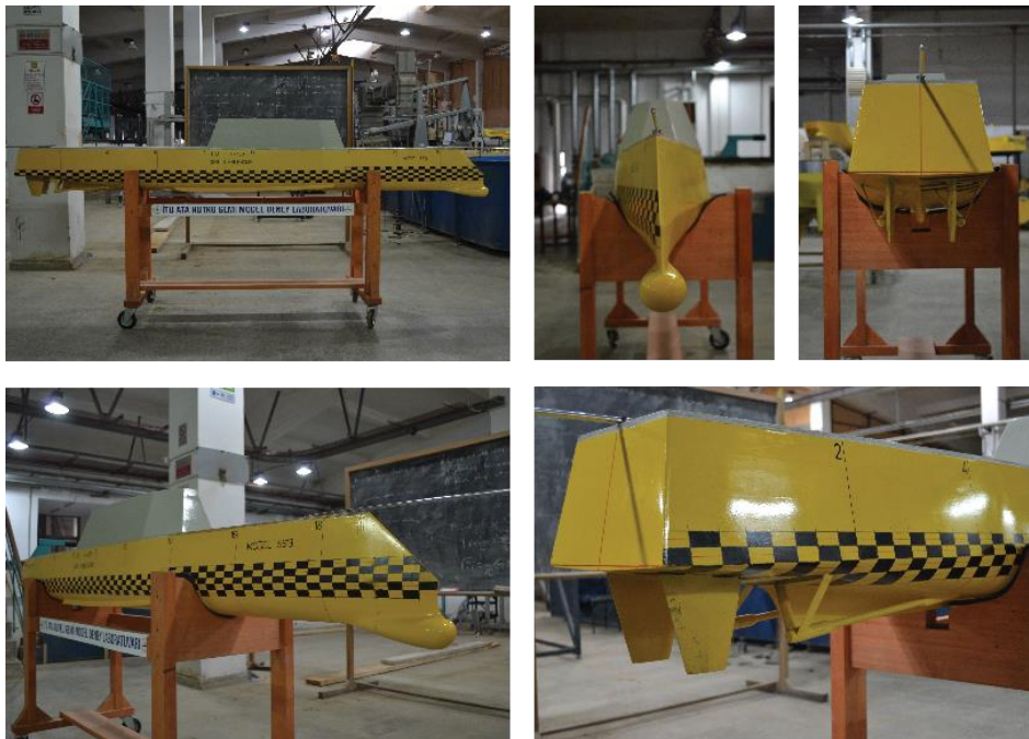
Figure 3.10 : 1/48.9 scaled ONRT model.
