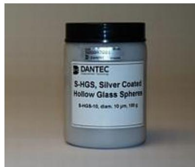
**Figure 2.12 :** Silver Coated Hollow Glass Particles.
