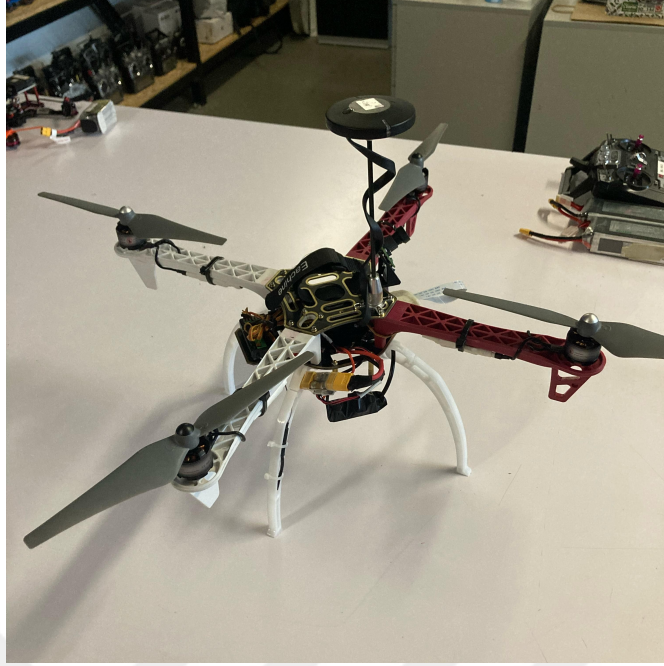
Figure 3.3: The small UAV prepared for the flight tests carrying down-facing onboard camera and IMU
