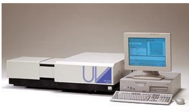
Figure 5.3 : UV – vis – NIR spectrophotometer (SHIMADZU UV-3150).
