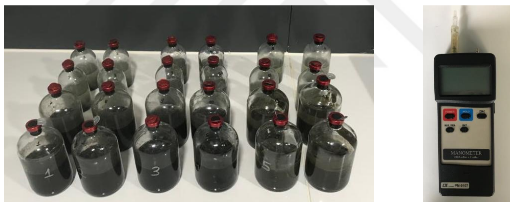
Figure 4.7 : Reactor set-up for SMA batch tests and manometer.
