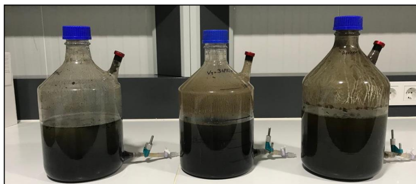
Figure 4.6 : Reactor set-up for biochemical methane potential tests.
