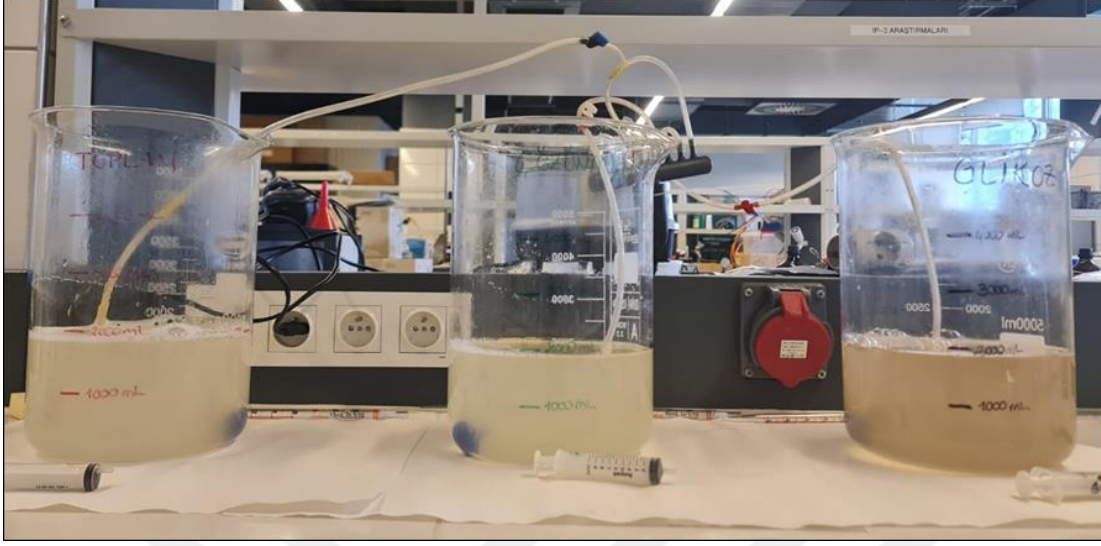
Figure 4.2 : Reactor set-up for identification of inert COD fractions.
