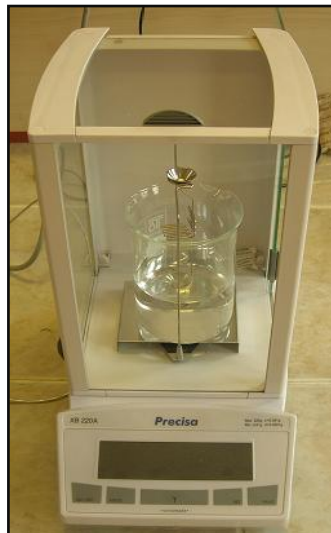
Figure 4.8: Precisa™ XB220A weighing machine and the Archimedes method mechanism
