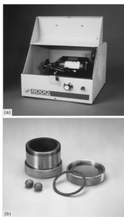
Figure 2.4: a) A typical Spex shaker mill b) Tungsten carbide vial set consisting of the vial, lid, gasket, and balls (Suryanarayana, 2001).
