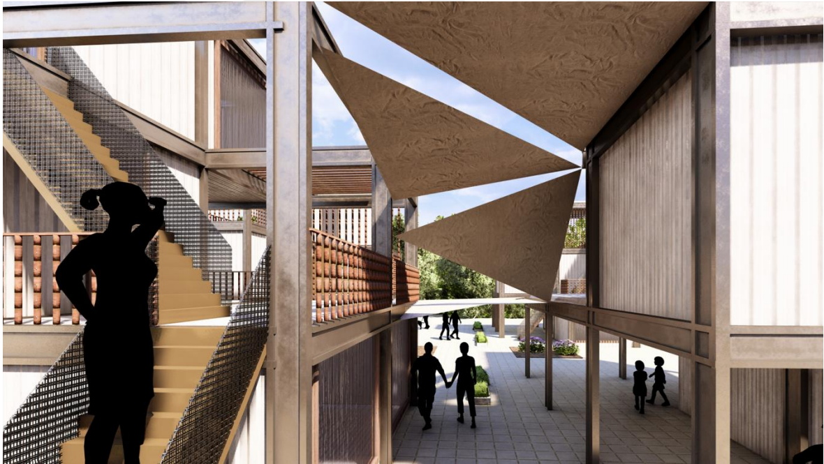
Figure A.5: Fabric sunshades between modules.
