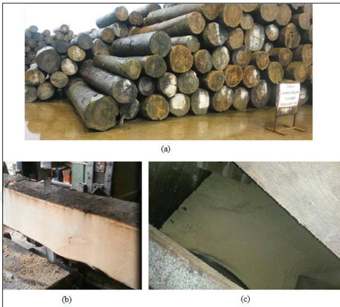
Figure 3.2 : Collection of industrial wood sawdust samples from Inegol region: (a) Logs (b) Cutting section (c) Sawdust wells.
