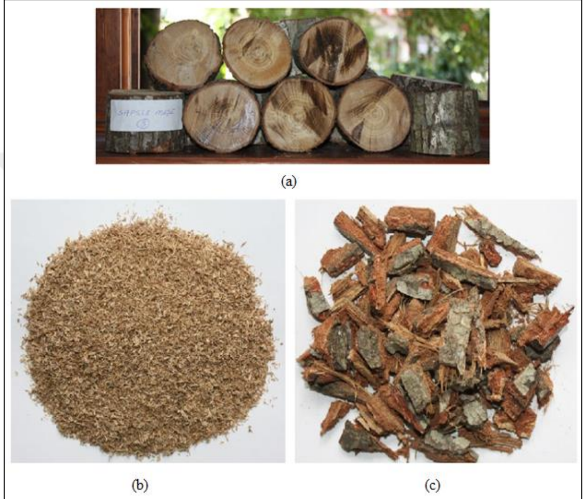
Figure 3.1 : Sessile oak ( Quercus petraea ) samples: (a) Logs (b) Meshed wood (c) Bark.
