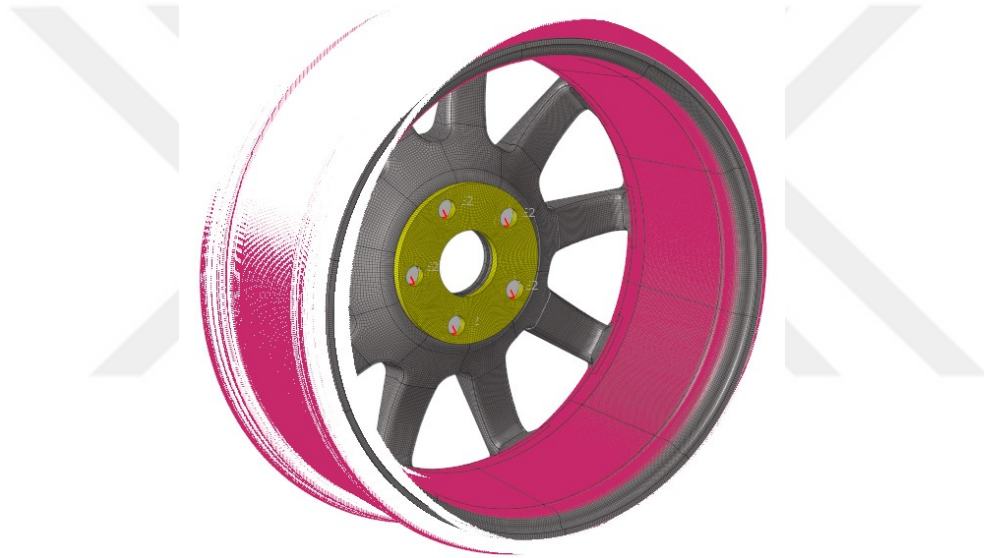
Figure 5.10 : Radial load case inflation pressure loading.
