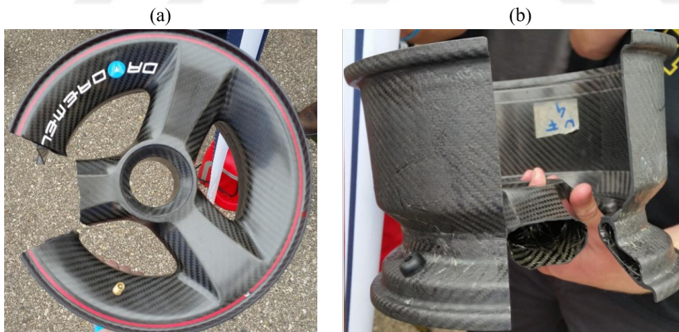
Figure 1.2 : Graz's composite rim: (a)Rim. (b)Section of rim [2].
