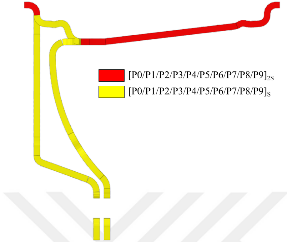
Figure 6.2 : Input parameters for layup.
