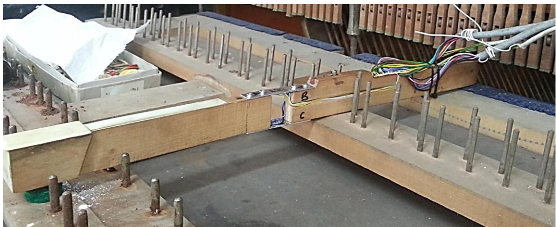
Figure 3.15 : Prototype key installed in piano.
