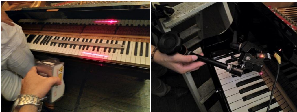
Figure 3.28 : Stripe and point laser sensors with FOV problems
