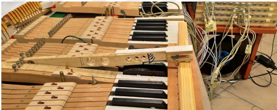
Figure 3.26 : Holes for weight balancing leads.
