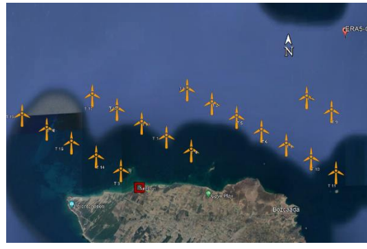
Figure 7.2 (continued) : Layouts for offshore alternative scenarios: (c)16 WTGs. (d)20 WTGs.
