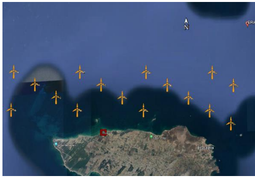
Figure 7.2 (continued) : Layouts for offshore alternative scenarios: (c)16 WTGs. (d)20 WTGs.
