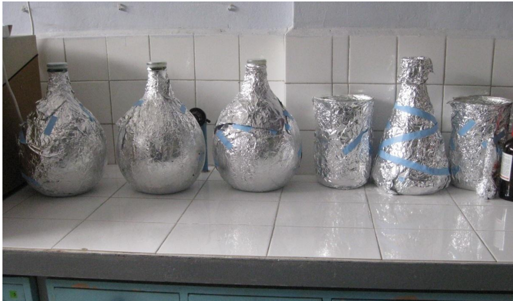
Figure 4.1 : Aluminum foil covered glass tanks
