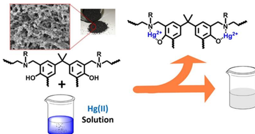
Figure 1 : Schematic illustration of mercury sorption mechanism.
