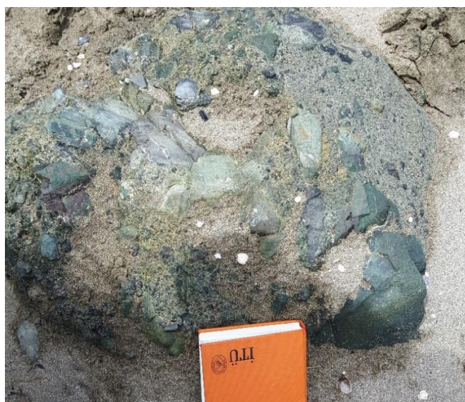
Figure 2.16 : Field photo of the poorly sorted andesitic and limestone blocks in the agglomerate from location 10.
