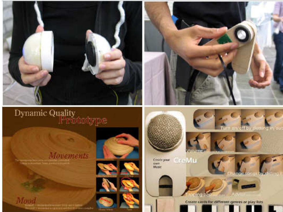
Figure 2.3.17: Top: interactive tangible sketches were produced within 3 hours, which were ‘fully’ working. Bottom: during several design cycles (including multiple 3D sketches) the sketches were transformed into interactive tangible prototypes, e.g. Cycles (left) and CreMu (right).
