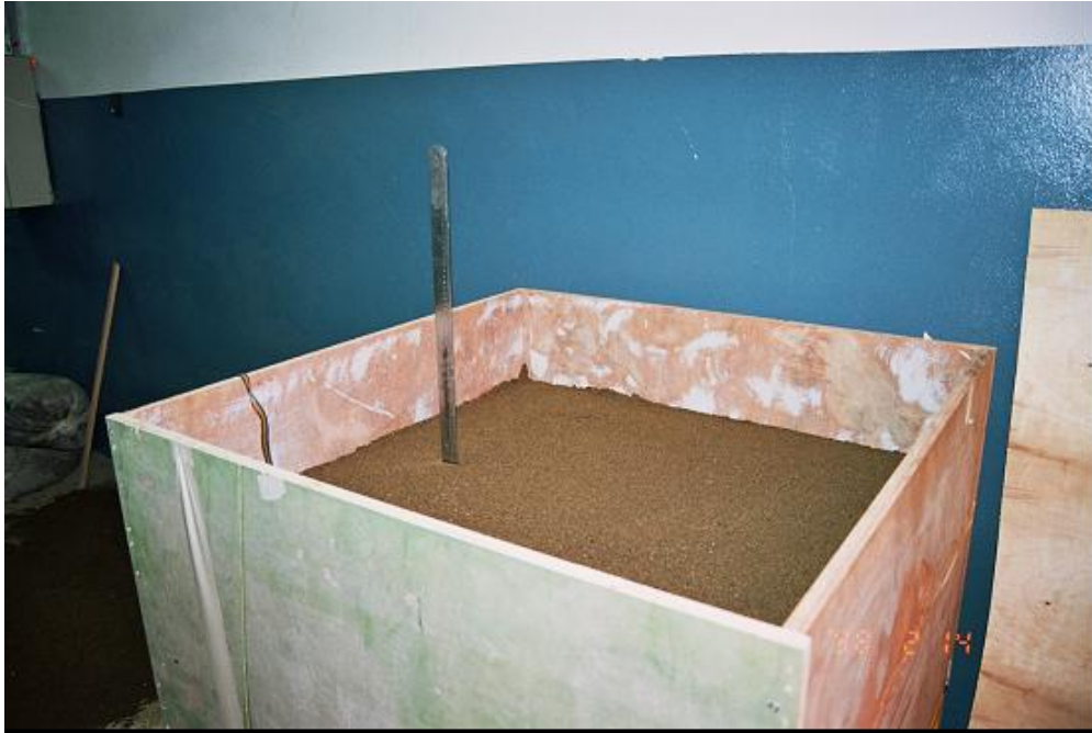
Figure M.12: The Sand Block at 450mm Height.
