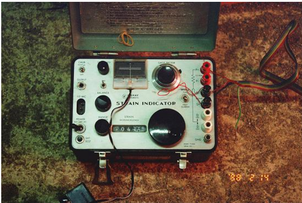
Figure M.13: The Strain Indicator.
