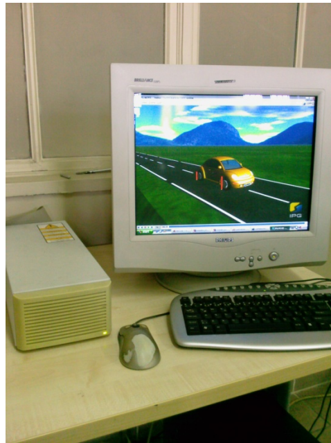
Figure 5.40 : DS1005 hardware and CarMaker screenshot.
