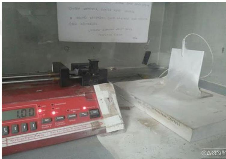
**Figure 3.1** : Photograph of the electrospinning set up.
