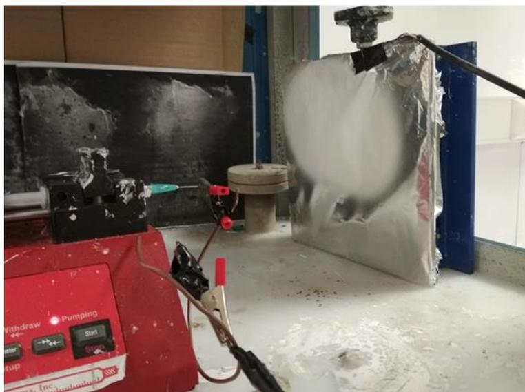
**Figure 4.3 :** Photograph of the electrospinning process.
