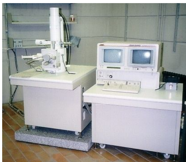
Figure 4.5 : JEOL™ JSM 5410 scanning electron microscope.
