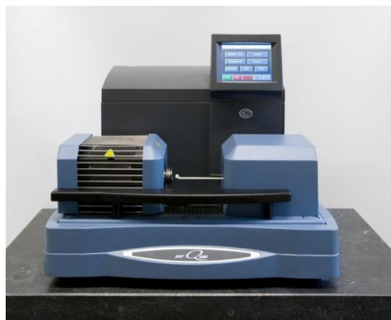
Figure 4.3 : TA™ Instruments Q600 DTA/TGA/DSC.
