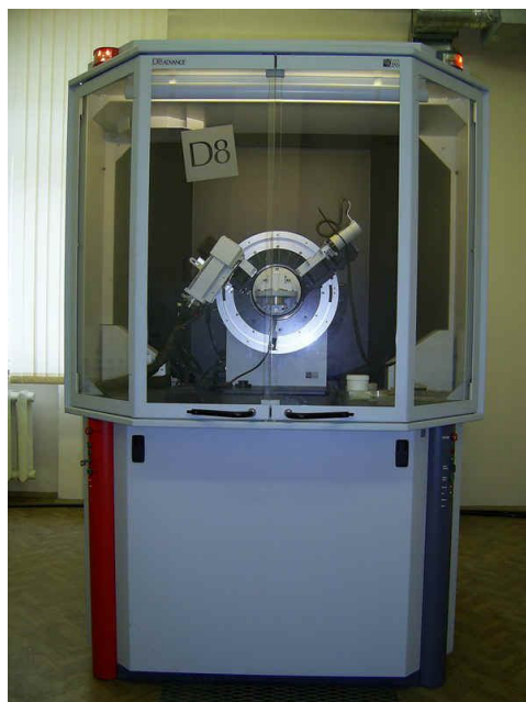
Figure 4.4 : Bruker™ D8 Advanced Series powder diffractometer.
