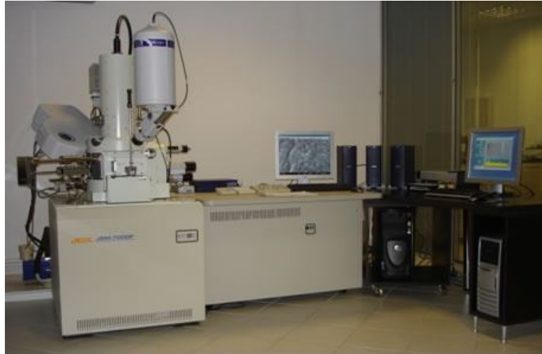
Figure 4.6 : JEOL JSM 7000F Field Emission Scanning Electron Microscope.
