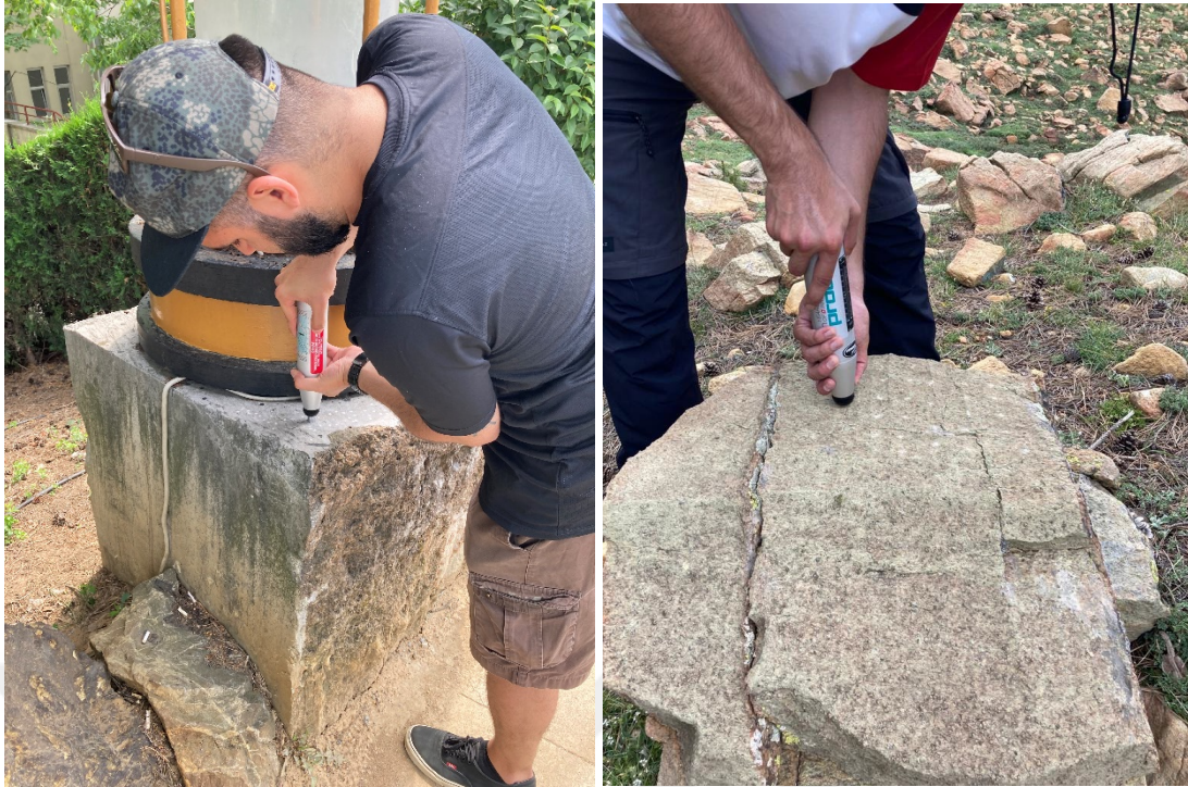
Figure A.3 : Measuring the marble calibration boulder located in front of the Faculty of Mines, Istanbul Technical University, Turkey (left), and a control boulder (SA22-617-SH) from the B2 moraine of the Northwest Valley, Mt. Sandıras (right).
