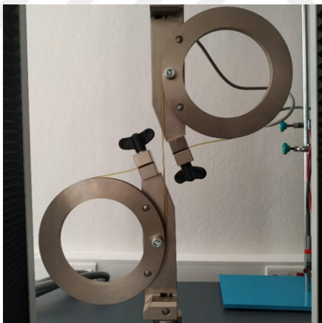
Figure 5.6 : An image from a neat PEI filament tensile test using SHIMADZU AGS-X UTM.
