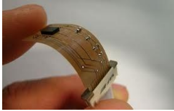
Figure 1.2: Flexible electronics for integration in a wearable textile system [3].
