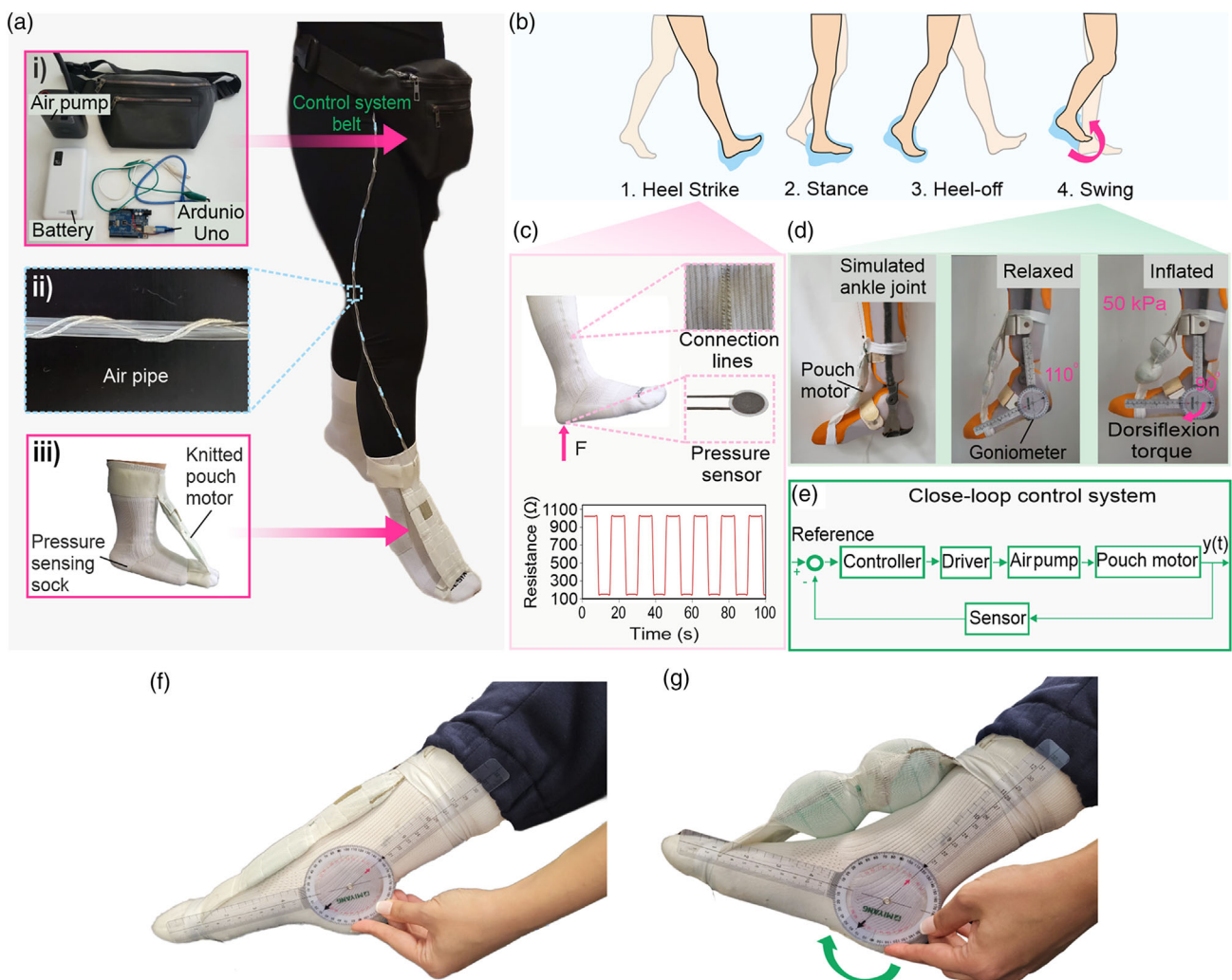
Figure 6. Application demonstration of the soft pouch motor in assistive robotics. a) Showing the concept behind the soft ankle-foot orthosis exosuit. b) Phases of the human gait. c) Functionality and application of the textile-based resistive pressure sensing sock. d) Dorsiflexion motion of the simulated ankle joint by soft pouch motor. e) Close-loop control block diagram. f) Deflated pouch motor fastened to a human foot. g) Dorsiflexion of the human foot using pouch motors that is inflated.
