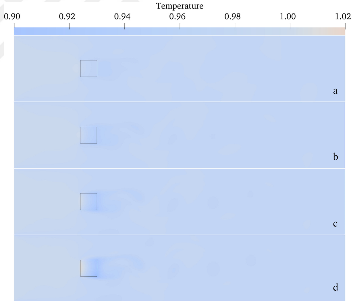
Figure 4.14 : Instantaneous contours of temperature distribution at Pr = 0.71 and k_r = 50 with varying Re : a) 50 b) 100 c) 150 d) 200.
