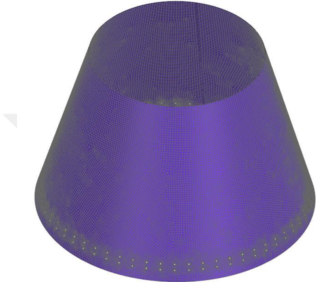
Figure 5.6 : General view of CFRP sandwich central coen FEM
