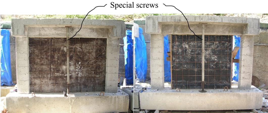
**Figure 3.8:** Specimens 6 and 7 having pre-reverse deflection on beam
