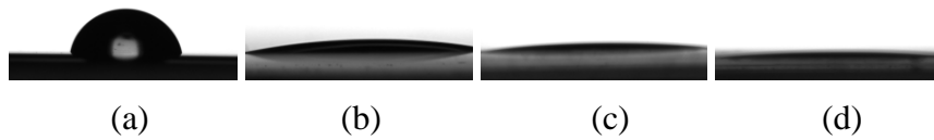
Figure 3.5 : Contact angle images of argon plasma treated Kapton HN films as a function of a duration (a) unmodified, (b) 1 min, (c) 3 min, (d) 5 min.
