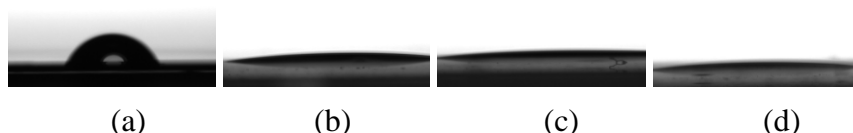
Figure 3.8 : Contact angle images of oxygen plasma treated Kapton TABE films as a function of a duration (a) unmodified, (b) 1 min, (c) 3 min, (d) 5 min.
