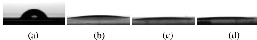
Figure 3.6 : Contact angle images of argon plasma treated Kapton TABE films as a function of a duration (a) unmodified, (b) 1 min, (c) 3 min, (d) 5 min.
