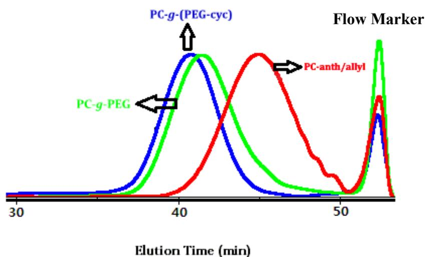
**Figure 4.17:** Overlay of GPC traces of PC-anth/allyl, PC-g-PEG, PC-g-(PEG-cyc) in THF at 30°C.
