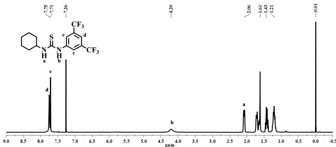
**Figure 4.2:** <sup>1</sup>H NMR spectrum of 1-(3,5-bis(trifluoromethyl)phenyl)-3-cyclohexylthiourea in CDCl<sub>3</sub> (500 MHz).
