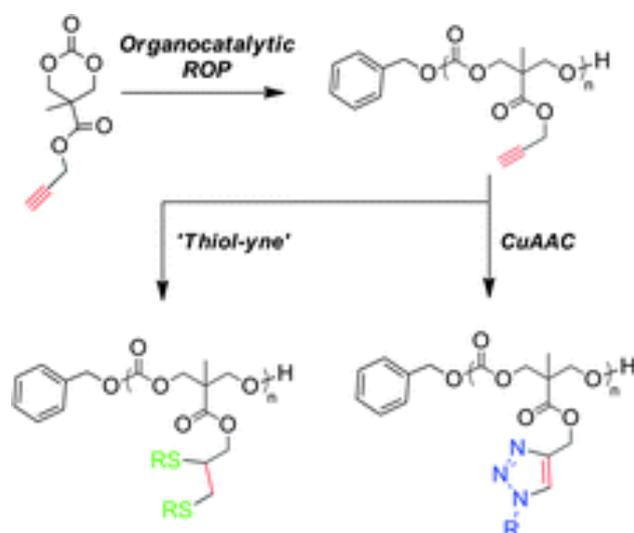
**Figure 2.17:** Propargyl-functional poly(carbonate)s via the organocatalytic ring-opening polymerization [157].
