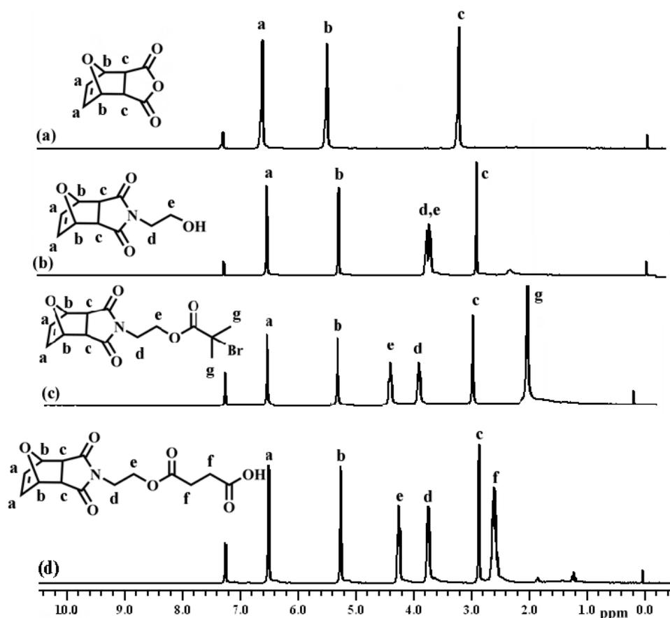
**Figure 4.1:**  $^1\text{H}$  NMR spectra of: a) 4,10-Dioxatricyclo[5.2.1.0<sup>2,6</sup>]dec-8-ene-3,5-dione (9); b) Synthesis of 4-(2-hydroxyethyl)-10-oxa-4-azatricyclo[5.2.1.0<sup>2,6</sup>]dec-8-ene-3,5-dione (10); c) 2-bromo-2-methylpropionic acid 2-(3,5-dioxo-10-oxa-4-azatricyclo[5.2.1.0<sup>2,6</sup>]dec-8-en-4-yl) ethyl ester (11); d) 4-(2-((3-acetyl-7-oxabicyclo[2.2.1]hept-7-yl)carbonyl)amino)ethoxy)-4-oxobutanoic acid (12) in  $\text{CDCl}_3$ .
