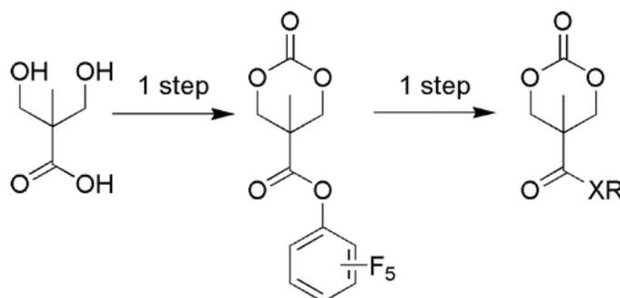
**Figure 2.13:** General synthetic route to functionalized cyclic carbonate monomers using pentafluorophenyl ester intermediate [154].
