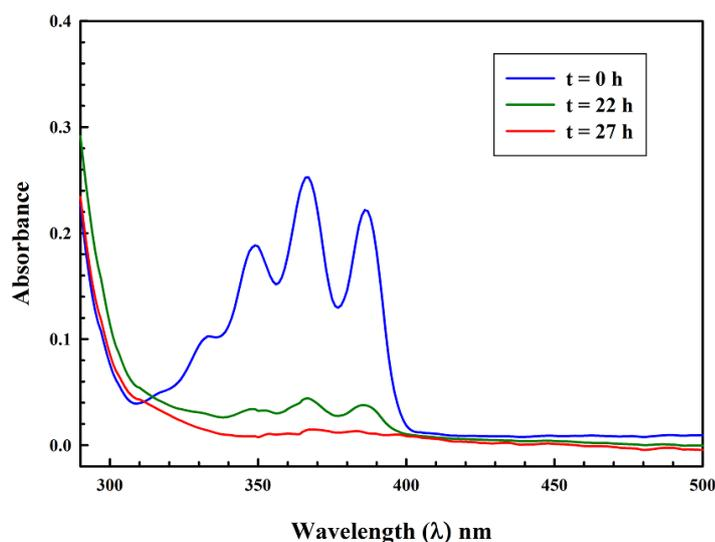
**Figure 4.14:** UV-Vis spectra of PC-g-PEG<sub>550</sub> copolymer ( $C_0 = 2.66 \times 10^{-5}$  M in  $\text{CH}_2\text{Cl}_2$ ).
