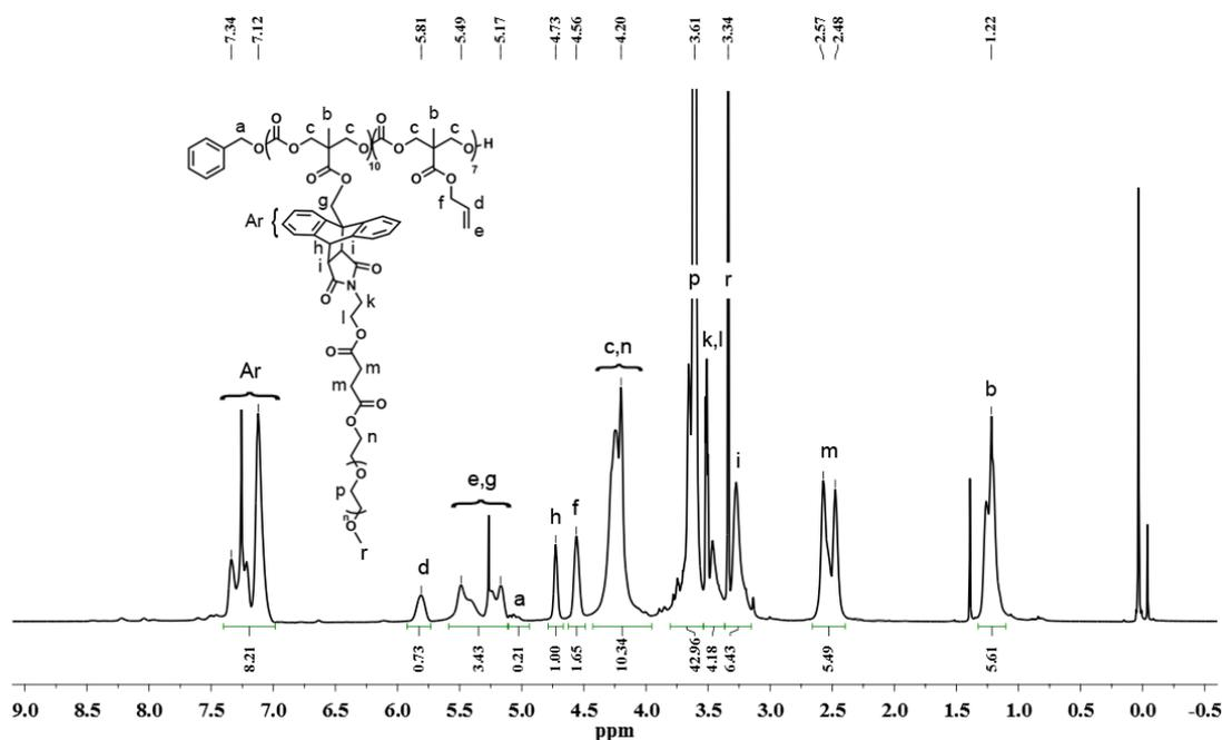
**Figure 4.15:**  $^1\text{H}$  NMR spectrum of PC-g-PEG copolymer (from PC-anthracene/allyl and PEG<sub>550</sub>-MI) in  $\text{CDCl}_3$  (500 MHz).
