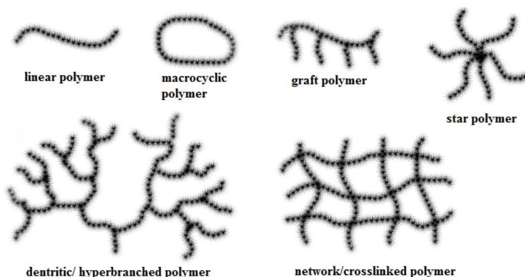
**Figure 2.8** Illustration of polymers with various topologies.
