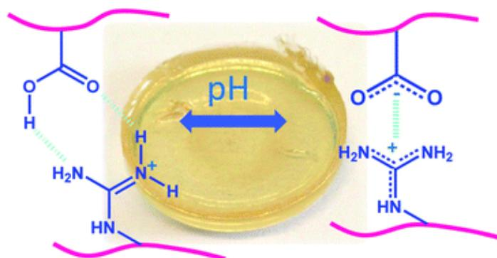
**Figure 2.16:** Bio-inspired stabilization of aliphatic polycarbonate-based hydrogels.
