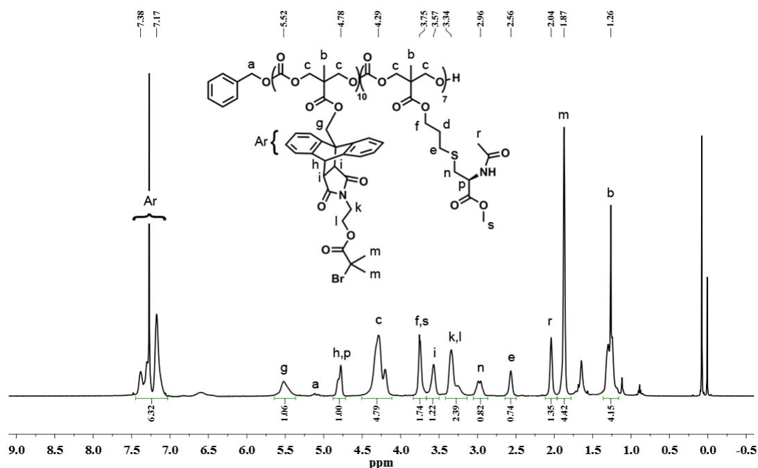
**Figure 4.11:**  $^1\text{H}$  NMR spectrum of thiol-ene click reaction of PC-g-MI with N-Acetyl-L-Cysteine Methyl-Ester (500 MHz).
