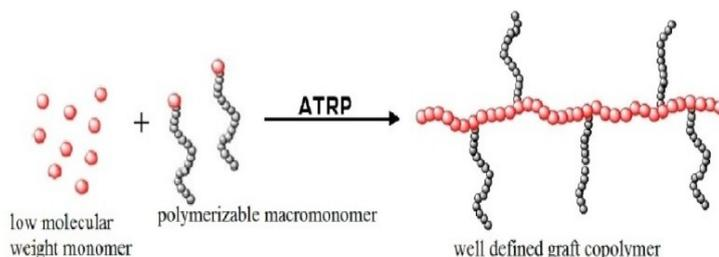
**Figure 2.9:** Synthesis of well-defined graft copolymer via grafting through method.
