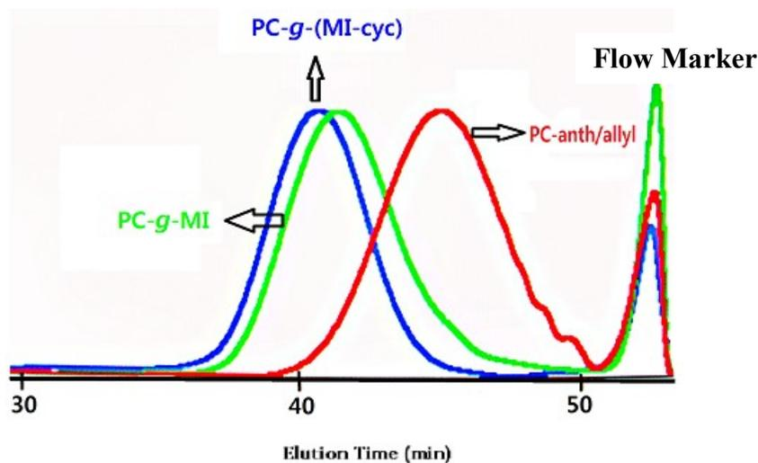
**Figure 4.12:** Overlay of GPC traces of PC-anth/allyl, PC-g-MI and PC-g-(MI-cyc) their block copolymers in THF at 30°C.
