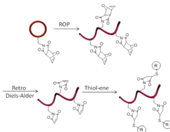
**Figure 2.18:** Illustrative scheme outlining the synthesis of maleimide containing polymers [158].
