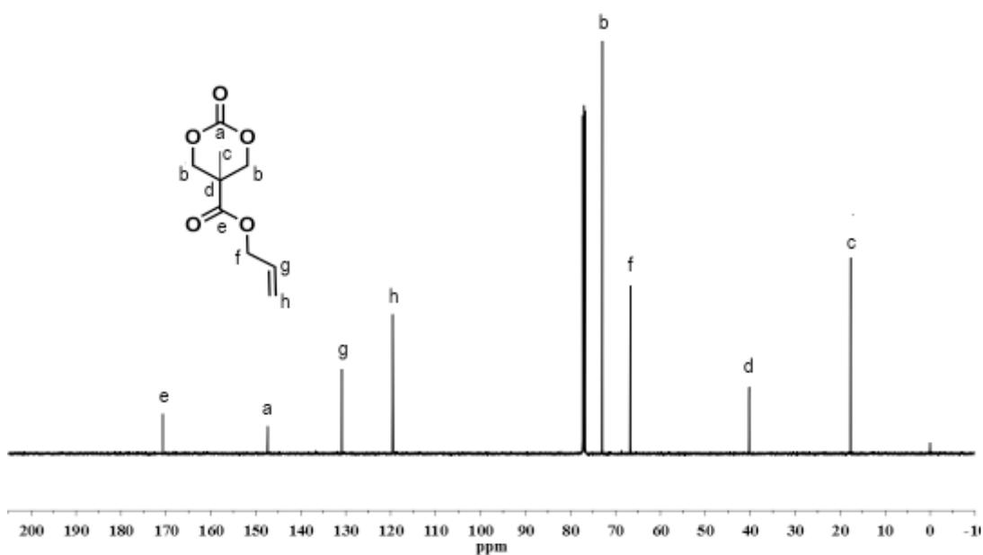
**Figure 4.6:**  $^{13}\text{C}$  NMR spectroscopy of Allyl-Carbonate in  $\text{CDCl}_3$  (500 MHz).
