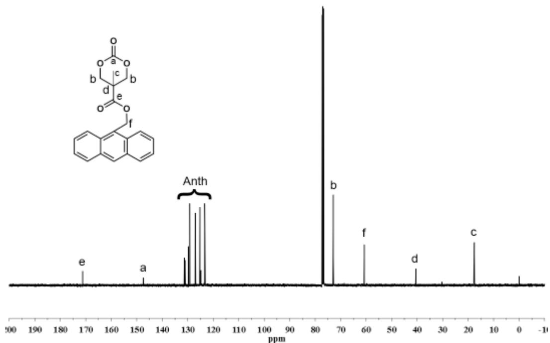
**Figure 4.4:** <sup>13</sup>C NMR spectrum of Anth-Carbonate in CDCl<sub>3</sub> (500 MHz).
