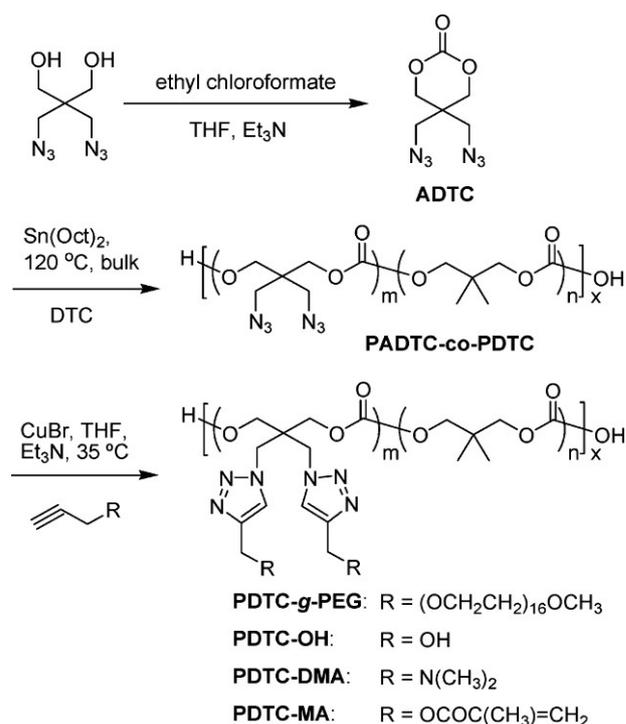
**Figure 2.14:** Synthesis of azido copolycarbonates PADTC-*co*-PDTC and their functionalization via the the click reaction [155].
