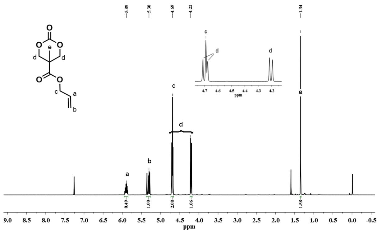
**Figure 4.5:**  $^1\text{H}$  NMR spectrum of Allyl-Carbonate in  $\text{CDCl}_3$  (500 MHz).
