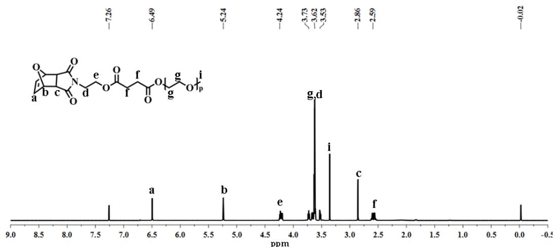
**Figure 4.13:**  $^1\text{H}$  NMR spectrum of PEG550-MI in  $\text{CDCl}_3$  (500 MHz).
