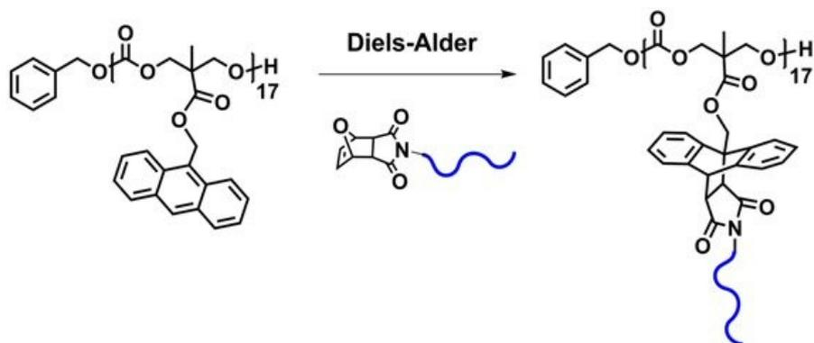
**Figure 2.11:** Diels–Alder click reaction for the aliphatic polycarbonate (PC) [19].
