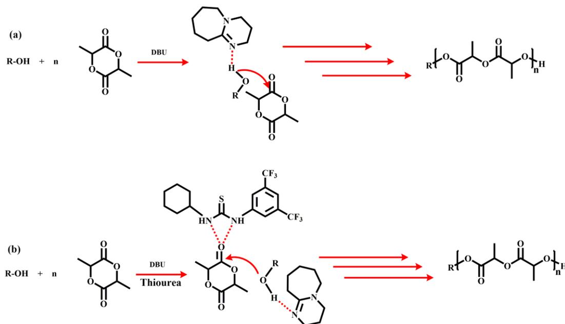
**Figure 2.7:** (a) Chain-end/general base activation in the presence of LA and DBU and (b) bifunctional activation of LA in the presence of ROH from an equimolar mixture of thiourea and DBU [113].
