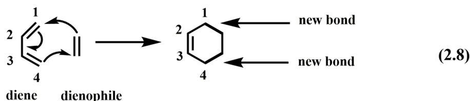
Typically, the DA reaction works best when either the diene is substituted with electron donating groups (like -OR, -NR<sub>2</sub>, etc) or when the dienophile is substituted with electron-withdrawing groups (like -NO<sub>2</sub>, -CN, -COR, etc) [117].
