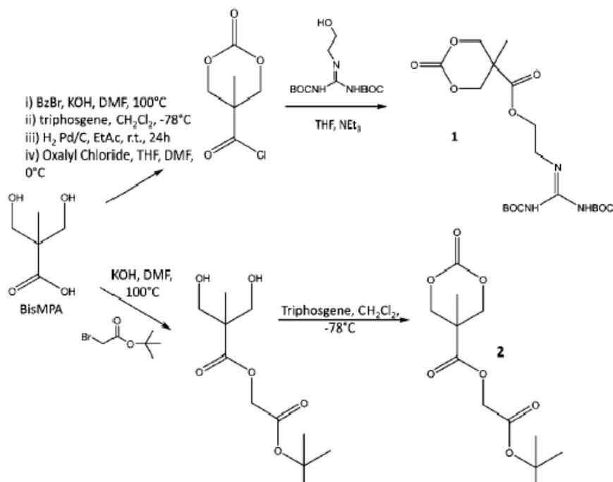
**Figure 2.15:** Synthesis of trimethylene carbonate-5-methyl-5-carboxyethyl guanidine 1,3-tert-butyloxy carbonyl (MTC-GuaBOC) and trimethylene carbonate-5-methyl-5-carboxy-tert-butylacetate (MTC tBAc) [156].
