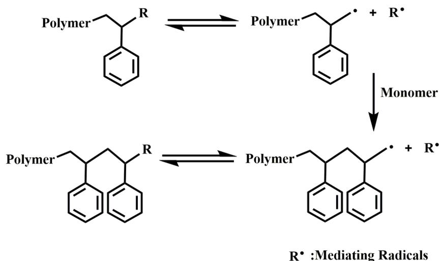
**Figure 2.1:** General mechanism of nitroxide mediated radical polymerization.
