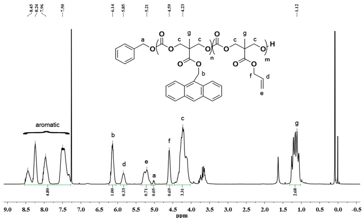
**Figure 4.8:**  $^1\text{H}$  NMR spectrum of benzyl-terminated polycarbonate (PC-anthracene and allyl) and cyclic carbonate in  $\text{CDCl}_3$  (500 MHz).
