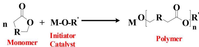
**Figure 2.2:** Schematic representation of the ROP of a cyclic ester  $R=(\text{CH}_2)_{0-3}$  and/or  $(\text{CHR})$ .
