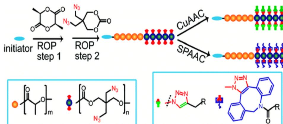
**Figure 2.10** : Synthesis of azido-functionalized polycarbonate via controlled/“living” ring-opening polymerization and functionalized with copper-catalyzed or copper-free strain-promoted azido-alkyne cycloaddition [93].
