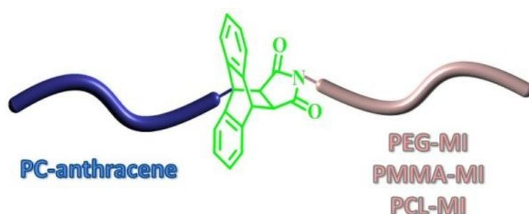
**Figure 2.12:** PC-based block copolymers (PC-*b*-PEG, PC-*b*-PMMA and PC-*b*-PCL) [153].
