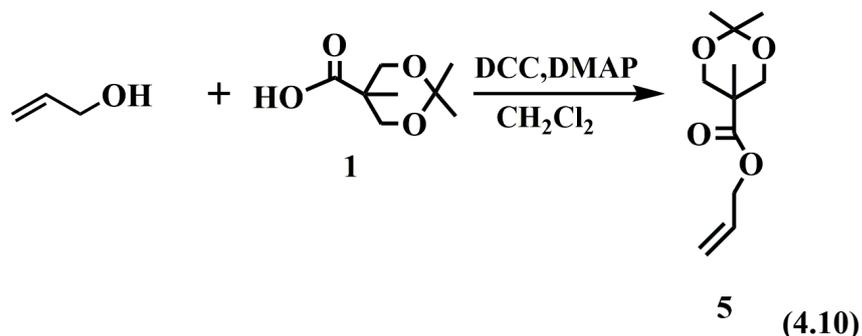
Next, (allyl 2,2,5-trimethyl-1,3-dioxane-5-carboxylate) **5** was hydrolyzed in THF by adding HCl solution stirring for 2 hours at room temperature.
