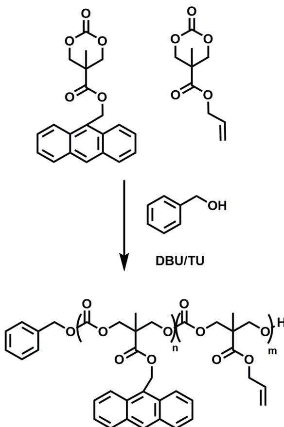
**Figure 4.7:** ROP of Anthracene and Allyl Functional Carbonate Monomers
