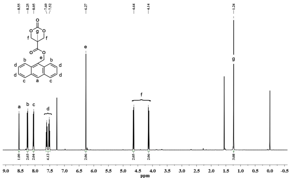
**Figure 4.3:** <sup>1</sup>H NMR spectrum of Anth-Carbonate in CDCl<sub>3</sub> (500 MHz).
