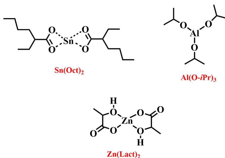
**Figure 2.3:** Catalysts of Ring Opening Polymerization.
