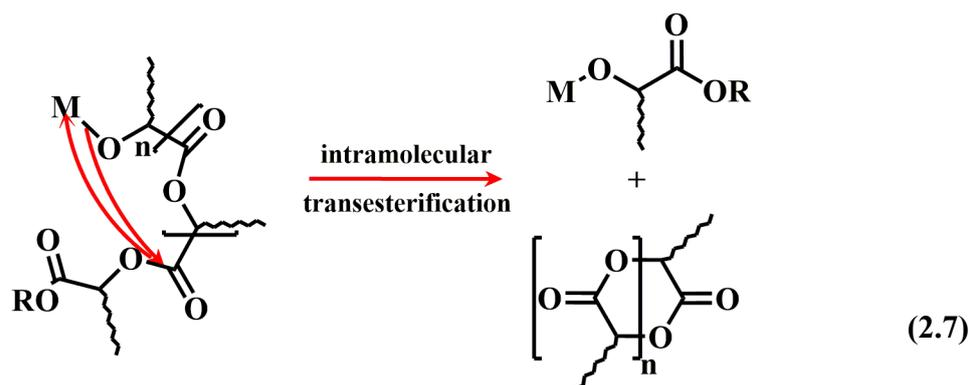
The promising results obtained with  $\text{Sn}(\text{Oct})_2$ ,  $\text{Al}(\text{Oi-Pr})_3$ , and  $\text{Zn}(\text{Lact})_2$  have given rise to a growing interest in metal-based initiators that would display higher catalytic activity and better control the extent of the undesirable transesterification reactions.
