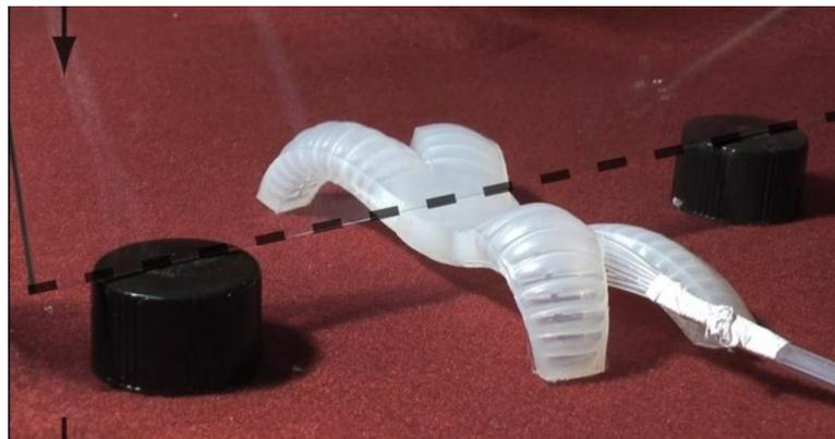
**Figure 1. 1 :** One of the Example of Multi-Gait Soft Robot. (Shepherd et al., 2011)
