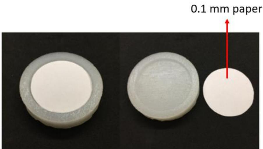
**Figure 4. 9 :** Strain Limiting Layer Assembly.
