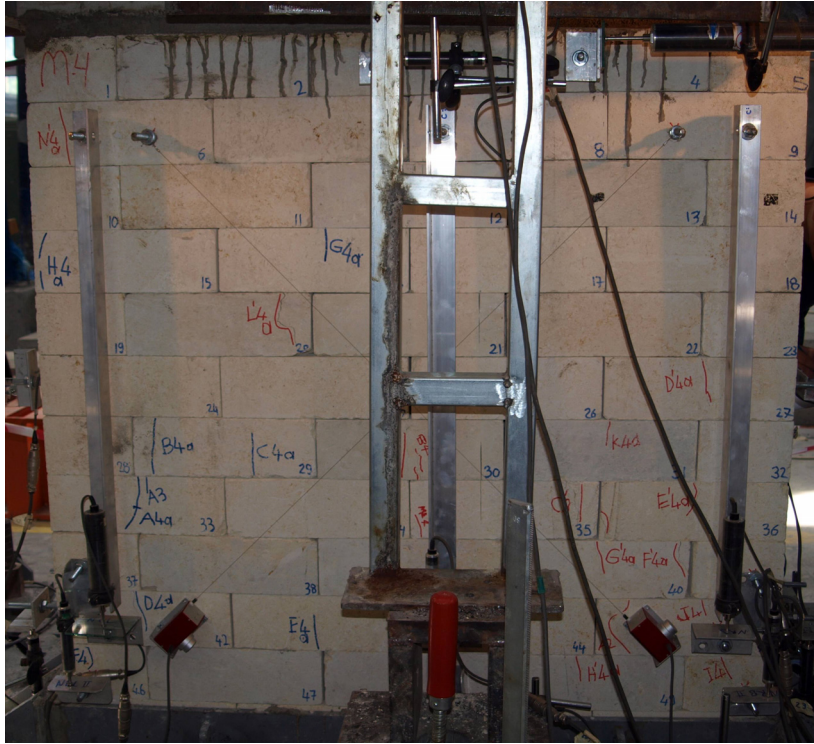
Figure C.119 : Cycle 4a, Northern face of M-50 after 0.50% drift ratio.
