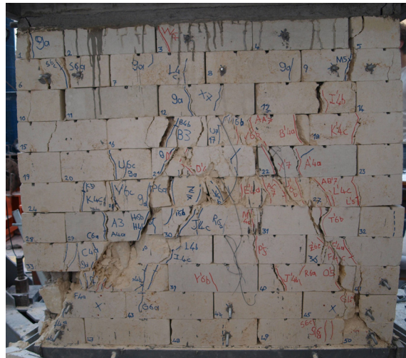
Figure C.181 : Northern face of M-50-CP after 2.0% drift ratio.
