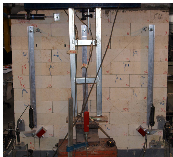
Figure C.87 : Cycle 2, Southern face of M-100-C after 0.10% drift ratio.
