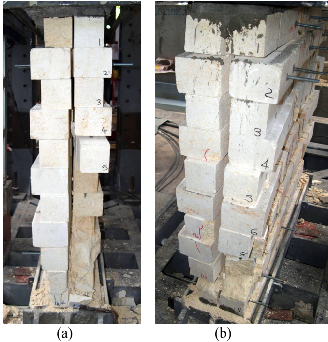
Figure C.157 : Cycle 8, (a) East and (b) West faces of S-50-C at the end of the test.
