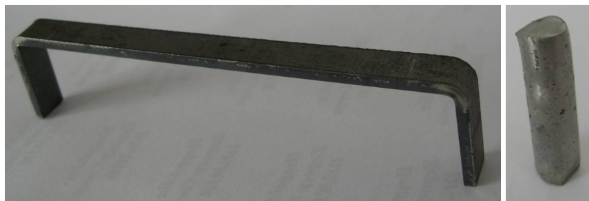
Figure 4.28 : Views of model cramp and pin reinforcements after production.
