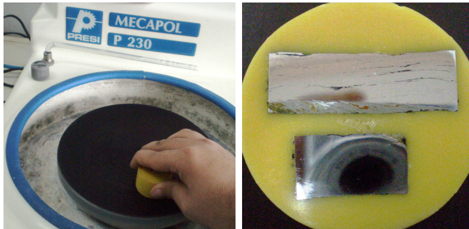
Figure 4.18 : Polishing of the metal sample surfaces.
