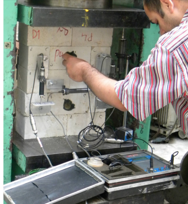
Figure 4.45 : Non-destructive ultrasound test on single-leaf prisms.
