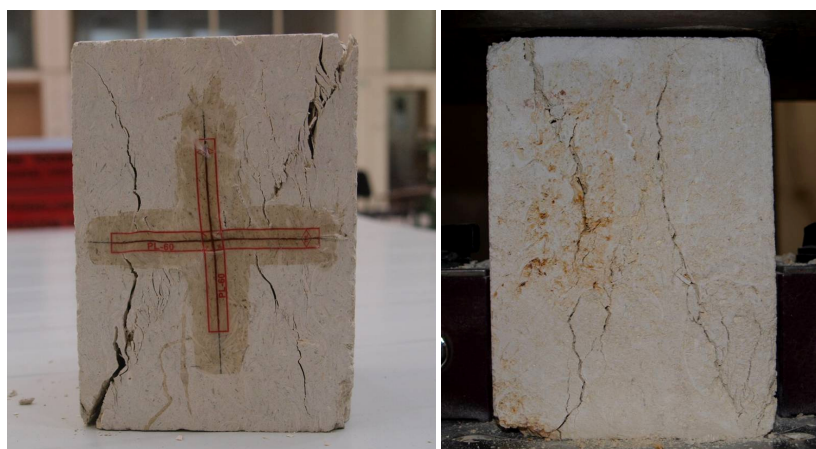
Figure 4.4 : Typical distribution of macro-cracks in single unit compression tests.
