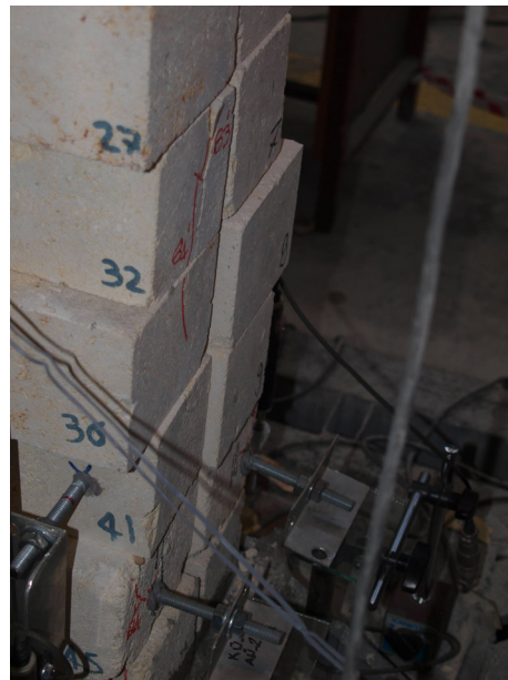
Figure C.149 : Sliding between the stone courses, S-50-C (0.75% drift ratio).
