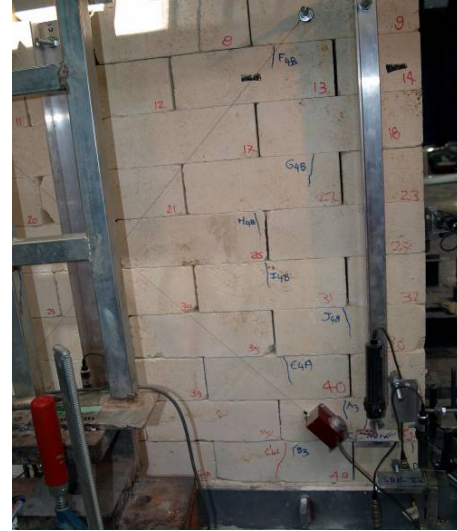
Figure C.35 : Cycle 4c, M-50-C after 5.50 mm displacement (0.50% drift ratio).
