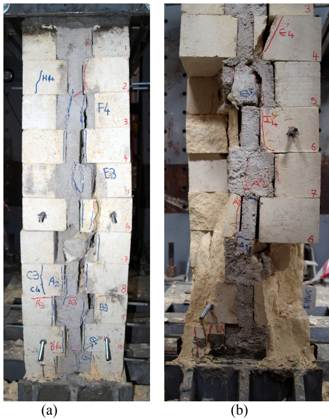
Figure C.133 : (a) Eastern and (b) Western faces of M-50 after the test.
