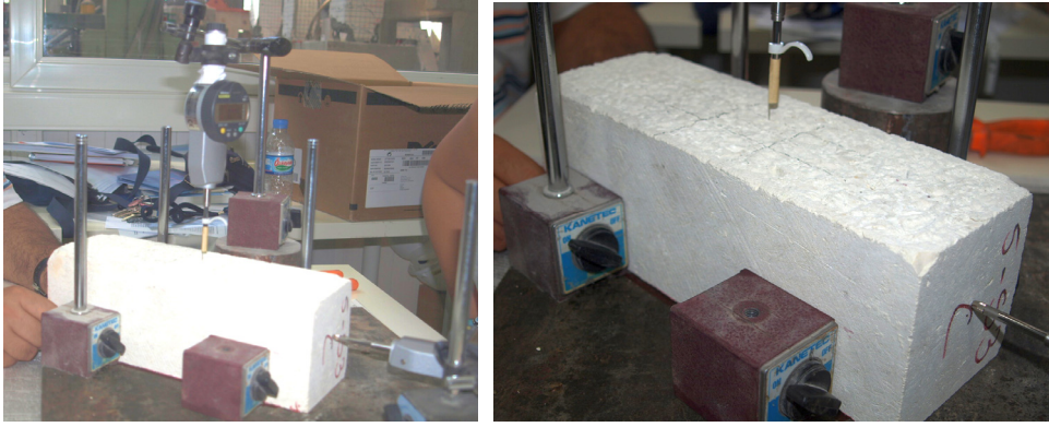
Figure B.1 : Stylus type profilometer developed for the current study.
