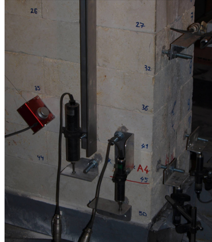
Figure C.61 : Cycle 4a, M-75-C after 5.50 mm displacement (0.50% drift ratio).
