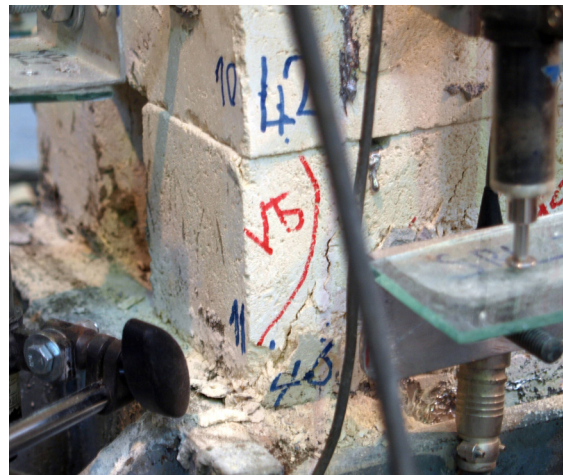
Figure C.201 : Cycle 5, S-50-C after 8.25 mm displacement (0.75% drift ratio).
