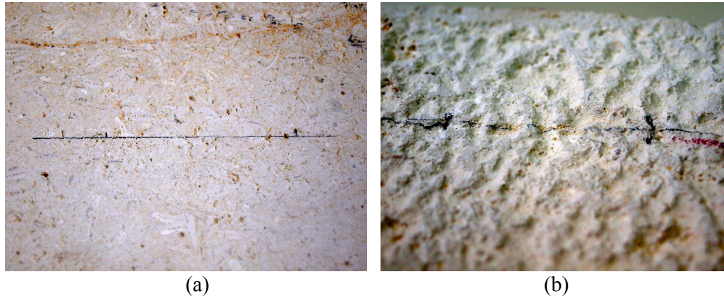
Figure 4.33 : Surface textures of SET I (a) and SET II (b) stone units.
