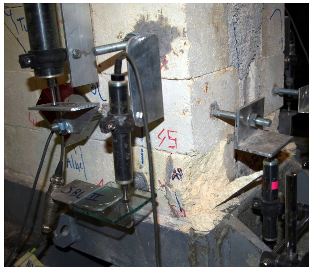
Figure C.95 : Cycle 5, toe crushing and spalling of M-100-C after 0.75% drift ratio.
