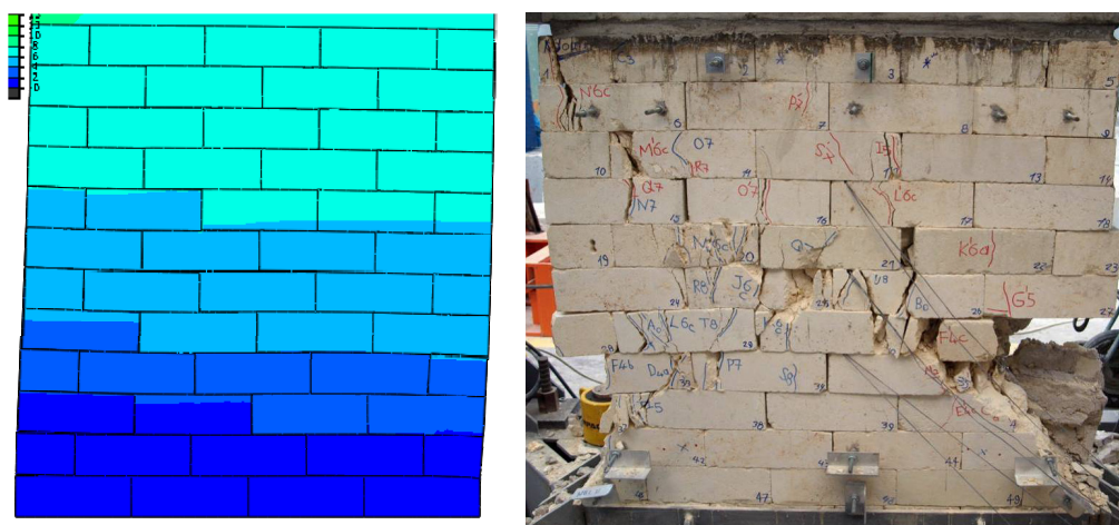
Figure 7.33 : Deformed shapes obtained from FEA and experiment (M-25-C).
