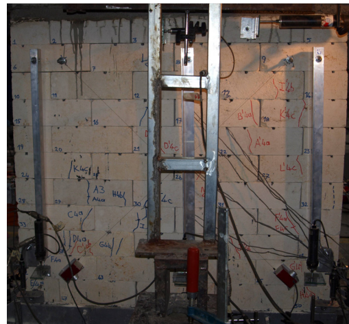
Figure C.173 : Cycle 4c, M-50-CP after 5.50 mm displacement (0.50% drift ratio).
