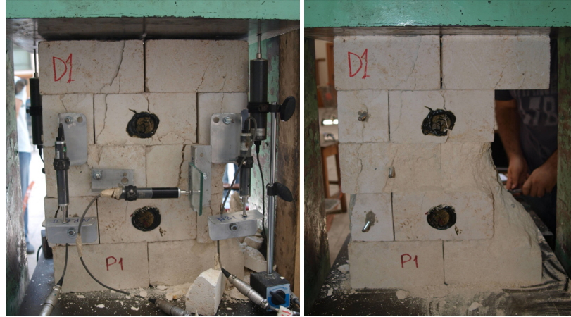
Figure 4.46 : Typical damage observed in the single-leaf prism compression tests.
