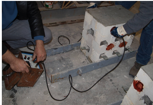
Figure 4.51 : Non-destructive ultrasound test on multi-leaf prisms.
