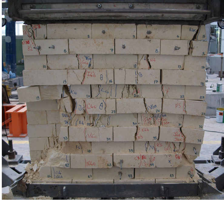
Figure C.155 : Cycle 8, North face of S-50-C at the end of the test.
