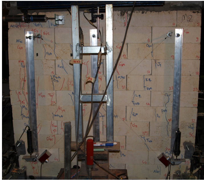
Figure C.94 : Cycle 4c, Southern face of M-100-C after 0.50% drift ratio.
