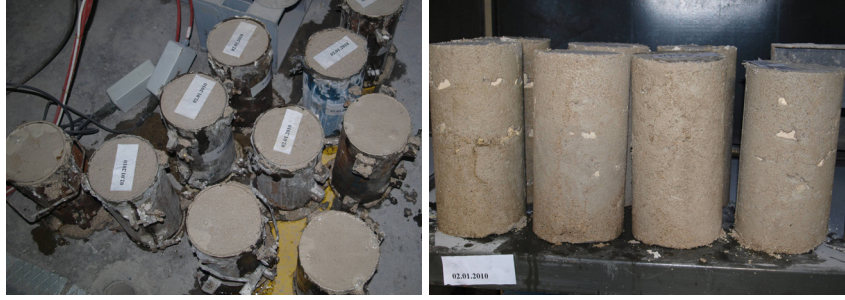
Figure 4.9 : Rubble masonry standard cylinder samples.
