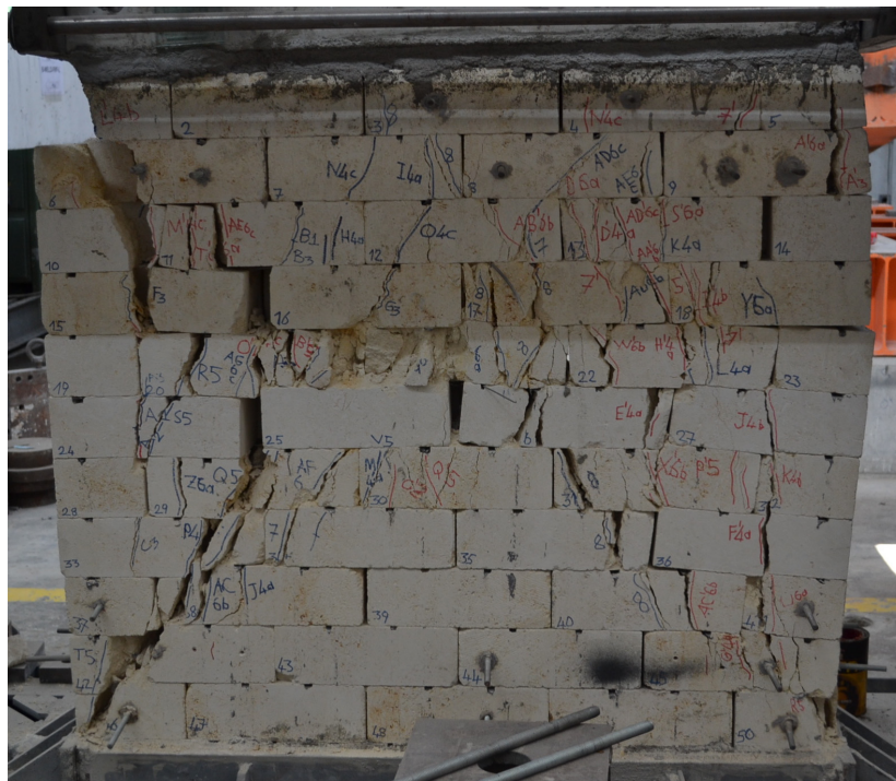
Figure C.208 : Cycle 9a, North face of S-50-CP after 1.50% drift ratio.
