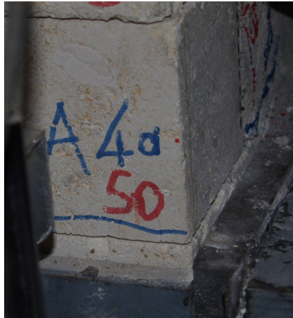
Figure C.62 : Cycle 4b, M-75-C after 5.50 mm displacement (0.50% drift ratio).
