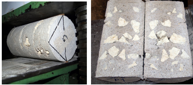
Figure 4.14 : The view of a typical specimen before and after the splitting test.
