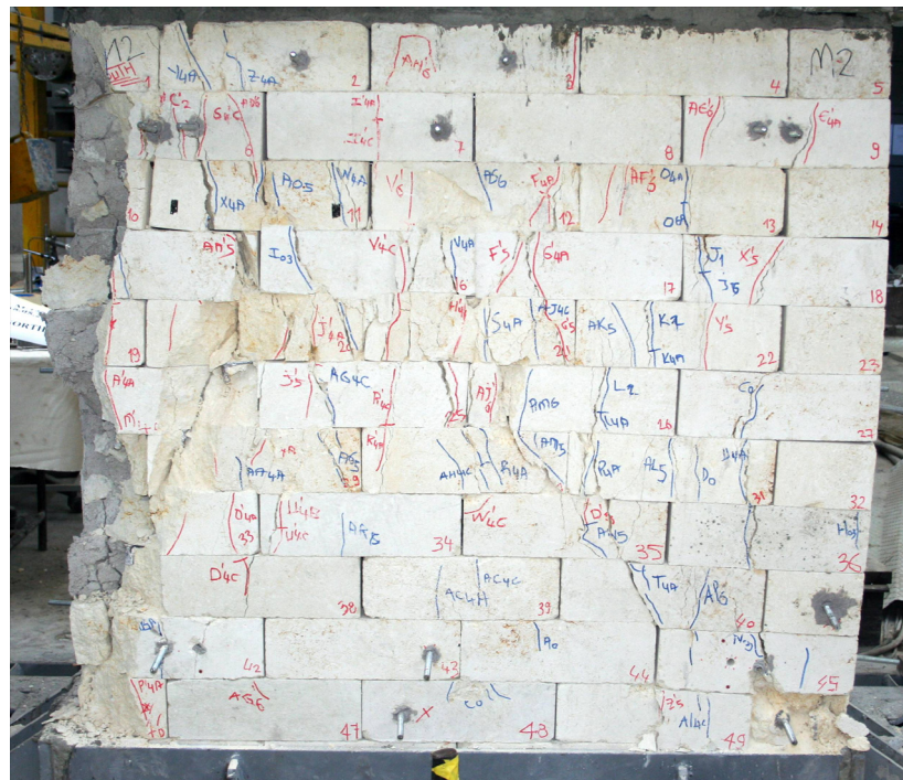
Figure C.101 : Southern face of M-100-C specimen after the test.
