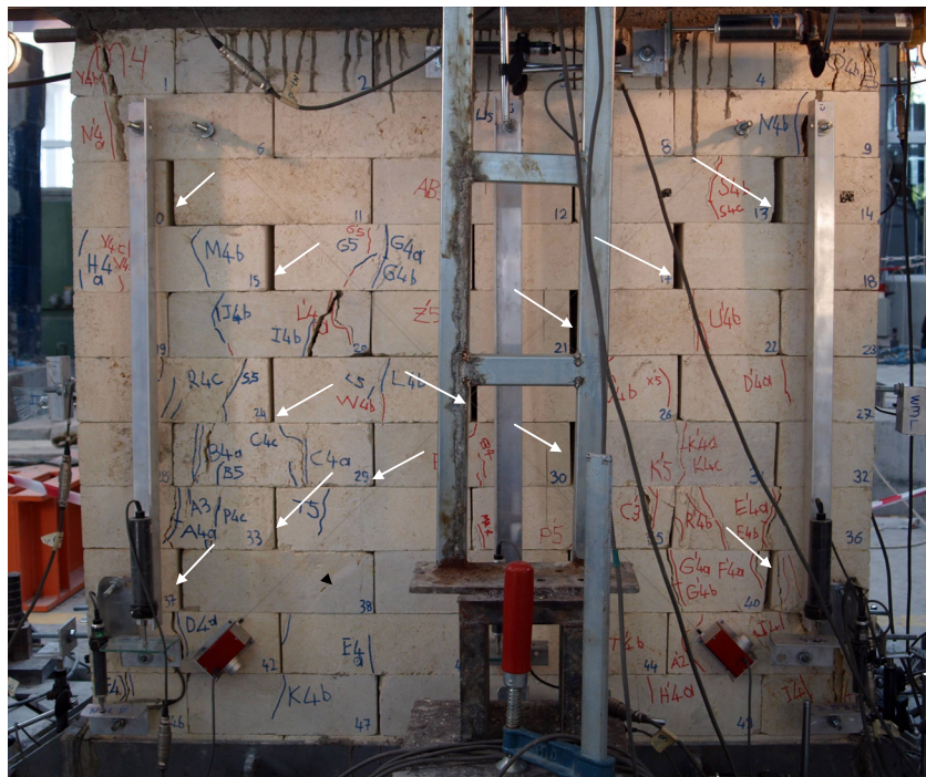
Figure C.124 : Cycle 5, Northern face of M-50 after 0.75% drift ratio.
