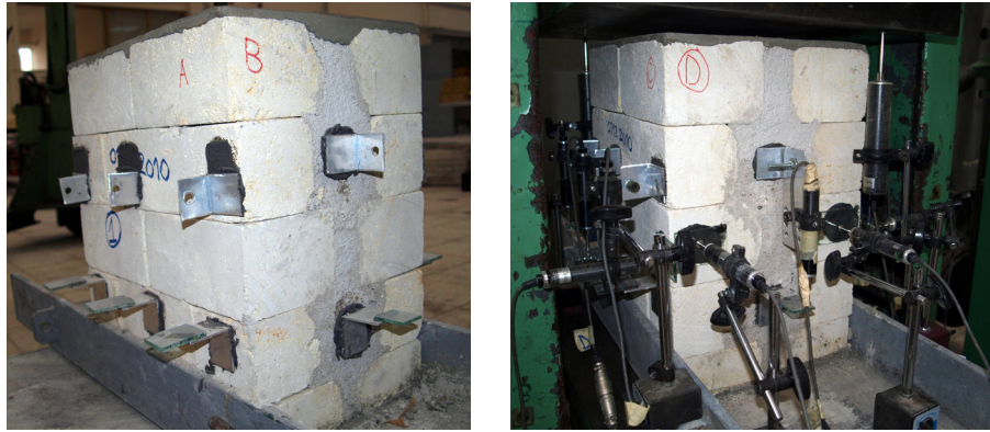
Figure 4.50 : Multi-leaf masonry prism before and after the instrumentation.
