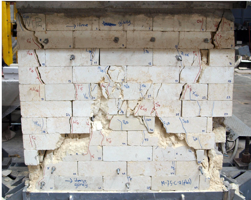
Figure C.72 : Cycle 7, South face of M-75-C (13.75 mm, 1.25% drift ratio).
