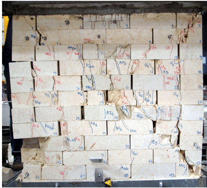
Figure C.132 : Southern face of M-50 specimen after the test.
