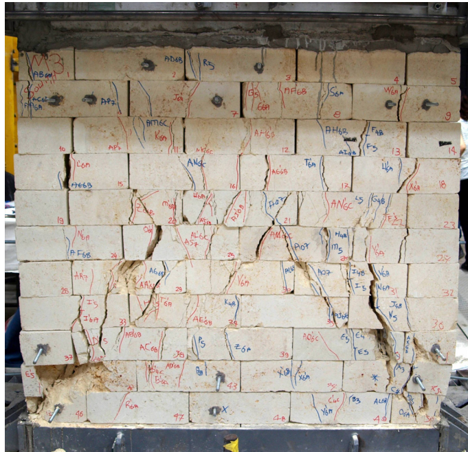
Figure C.43 : Cycle 8, South face of M-50-C after 1.50% drift ratio.
