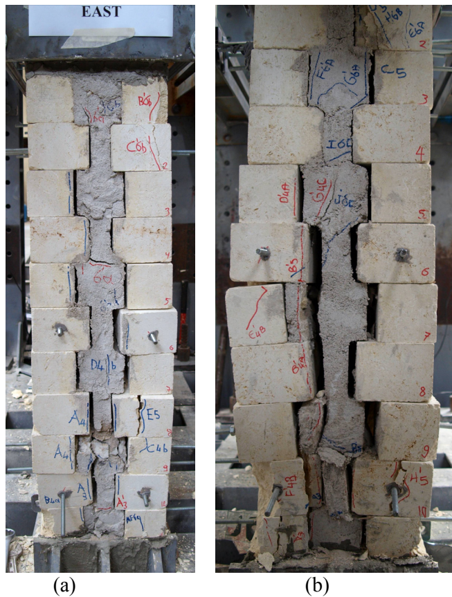
Figure C.44 : Cycle 8, (a) East and (b) West faces of M-50-C after 16.50 mm displacement (1.50% drift ratio).
