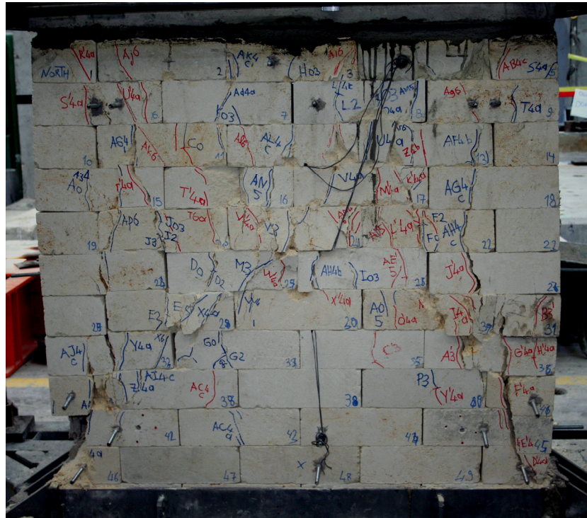
Figure C.100 : Northern face of M-100-C specimen after the test.
