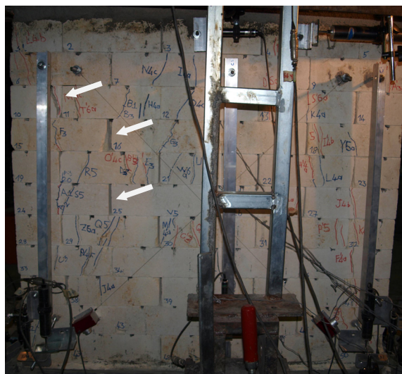
Figure C.202 : Cycle 6a, S-50-C after 11.0 mm displacement (1.00% drift ratio).
