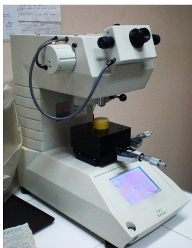
Figure 4.23 : Shimadzu HMV micro-hardness testing device used in this study.
