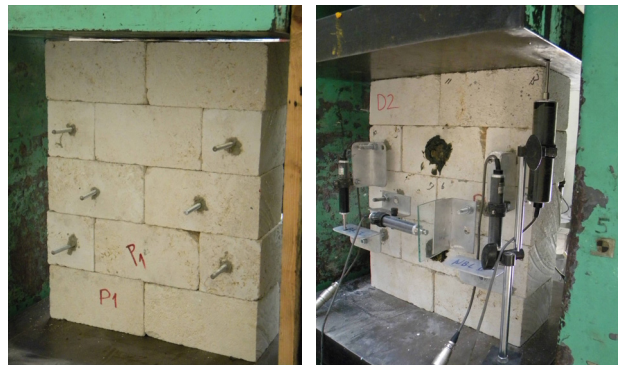
Figure 4.44 : Single-leaf masonry prism before and after the instrumentation.
