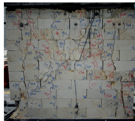
Figure 5.1 : Cracking patterns of M-25-C, M-50-C, M-75-C and M-100-C walls.
