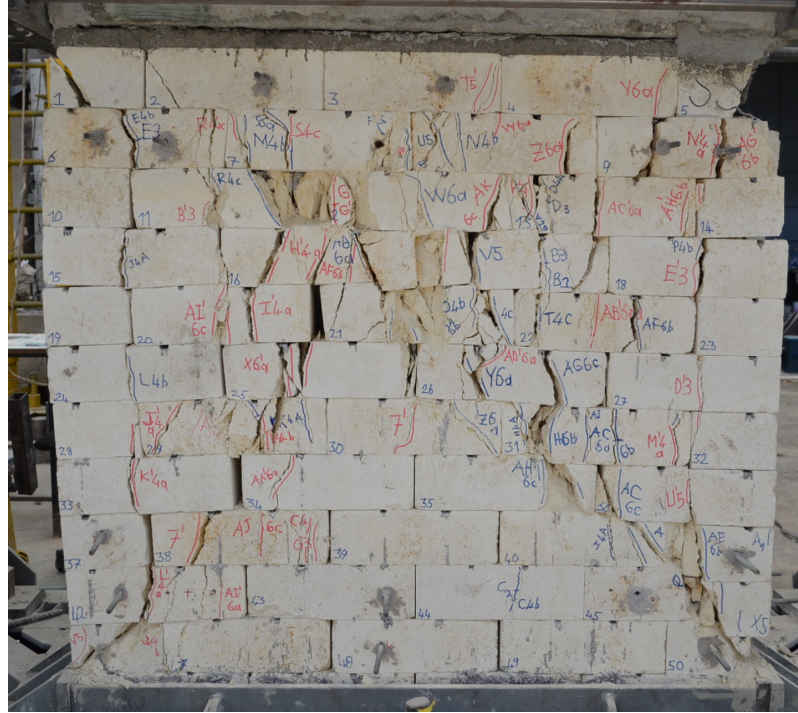
Figure C.209 : Cycle 8, South face of S-50-CP after 1.50% drift ratio.
