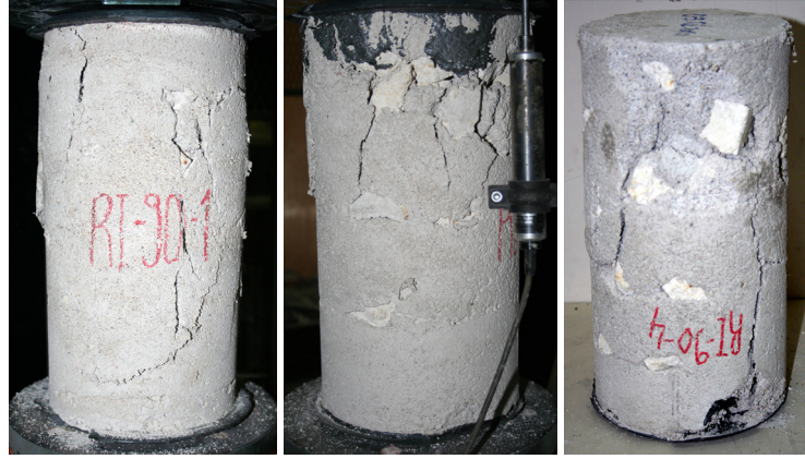
Figure 4.12 : The damage conditions of rubble masonry cylinders.
