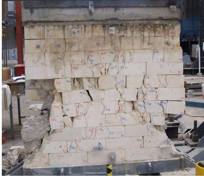
Figure C.16 : Cycle 9, South face of M-25-C after 2.0% drift ratio.
