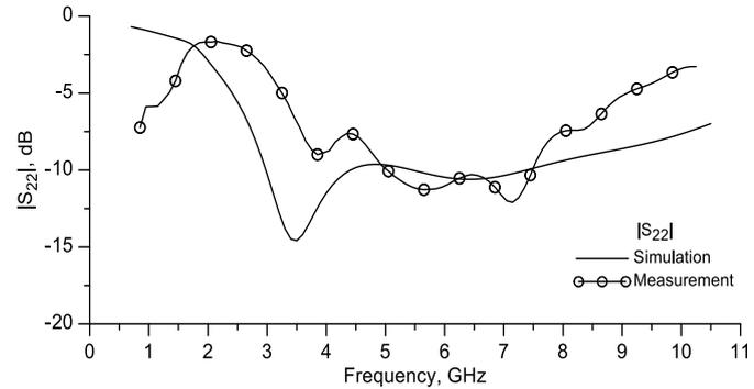
**Figure 4.46 :** The simulated and measured output matching ( $|S_{22}|$ ) performance of the DSTWPA.
