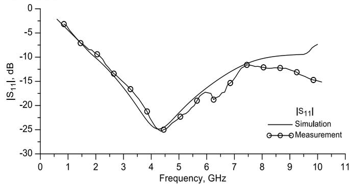
**Figure 4.45 :** The simulated and measured input matching ( $|S_{11}|$ ) performance of the DSTWPA.
